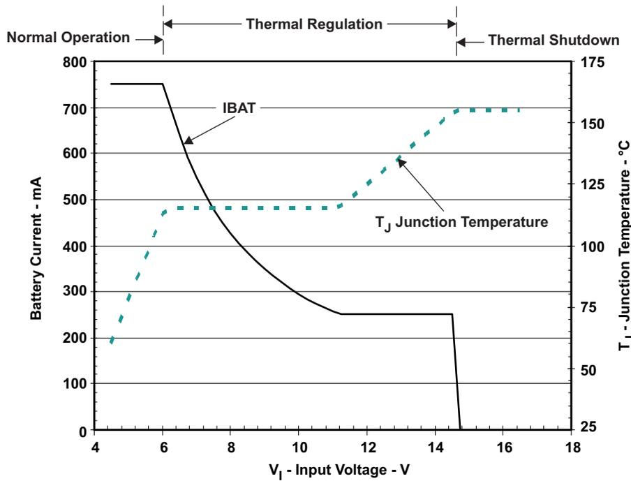
Figure 19. Thermal Regulation Loop Performance and Thermal Shutdown
