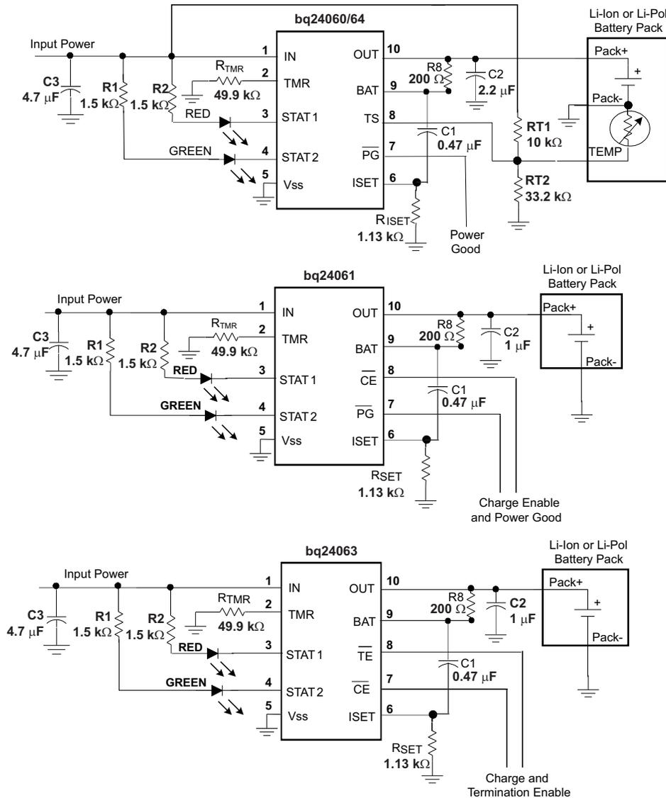
NOTE: Temp window set between 0°C and 45°C for application w/TS pin.
