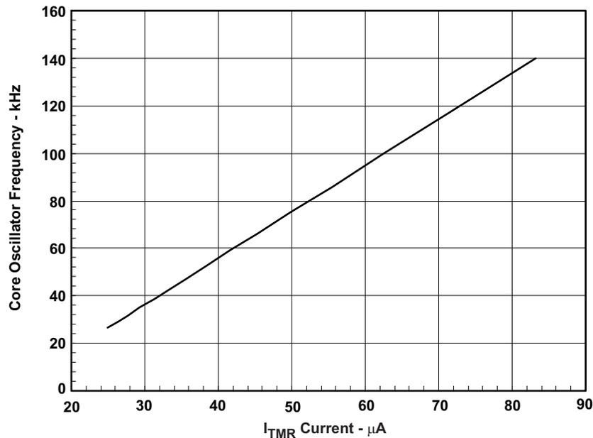
Figure 22. bq2406x Oscillator Linearity vs I<sub>TMR</sub>
