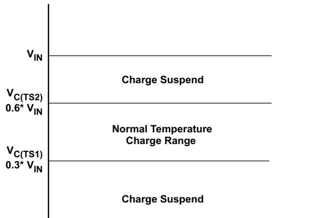
Figure 18. Battery Temperature Qualification With NTC Thermistor
