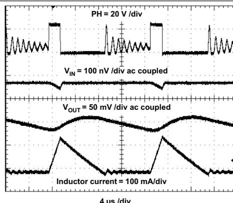
Figure 52. Input and Output Ripple in DCM
