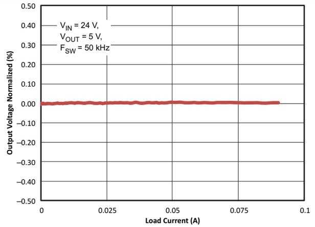
Figure 44. Output Voltage Normalized vs Load Current
