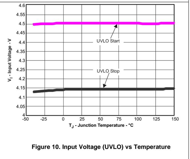
Figure 10. Input Voltage (UVLO) vs Temperature
