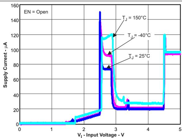
Figure 15. Supply Current (VIN Pin) vs Input Voltage (0 V to V<sub>START</sub>) En Pin Open
