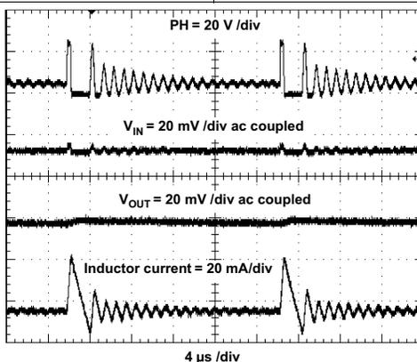
Figure 53. Input and Output Ripple in PSM
