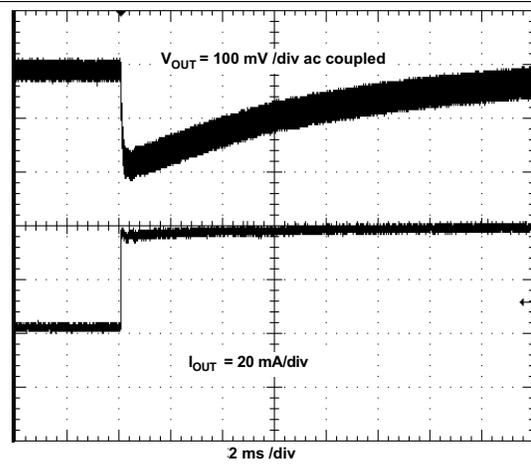
Figure 46. Load Transient
