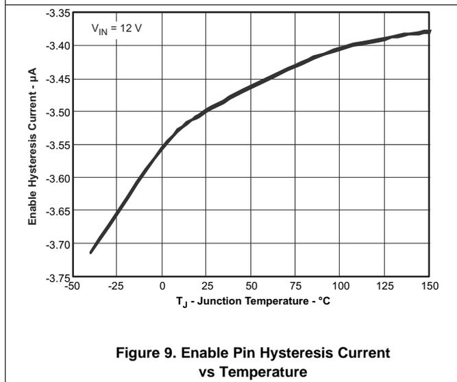
Figure 9. Enable Pin Hysteresis Current vs Temperature
