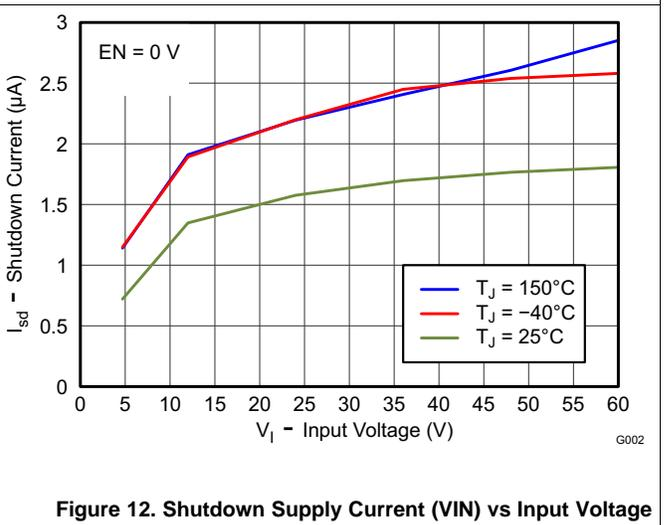
Figure 12. Shutdown Supply Current (VIN) vs Input Voltage
