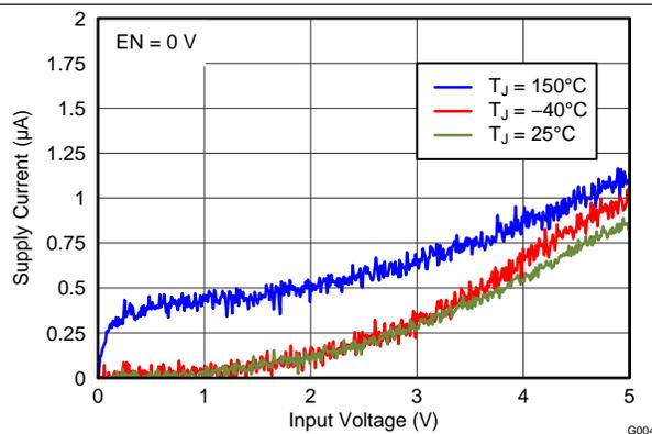
Figure 14. Supply Current (VIN Pin) vs Input Voltage (0 V to V<sub>START</sub>) En Pin Low
