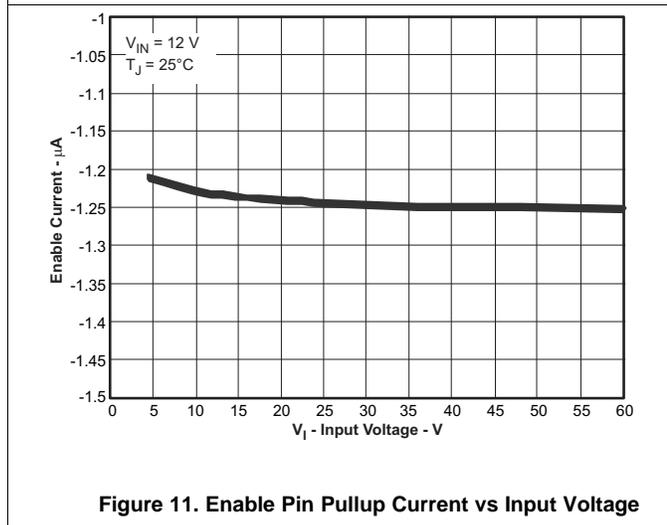
Figure 11. Enable Pin Pullup Current vs Input Voltage
