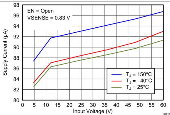
Figure 13. Supply Current (VIN Pin) vs Input Voltage
