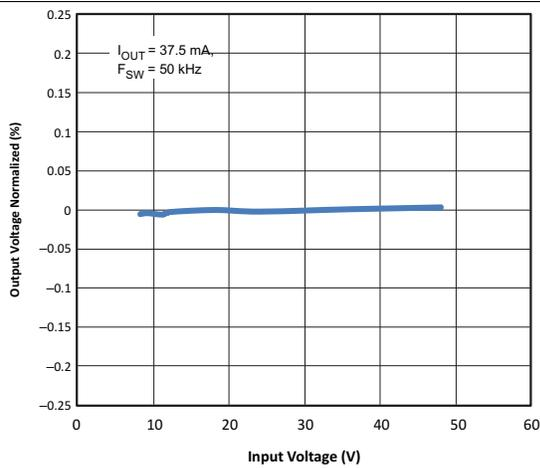
Figure 45. Output Voltage Normalized vs Input Voltage
