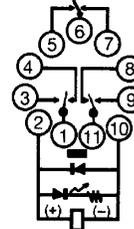
LED indicator and Varsistor type (AC coil)
