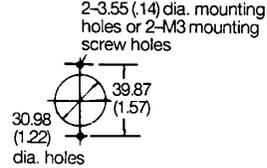
Mounting holes and panel cut-out applies to PL08 and PL08-Q
