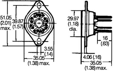
**Printed circuit board socket
