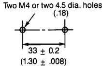
**Mounting dimensions of relay with socket**
