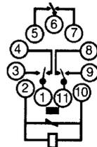
LED indicator and diode type (DC coil)
