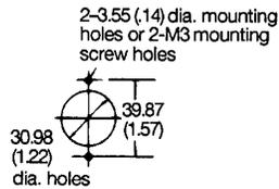
Mounting holes and panel cut-out applies to PL11 and PL11-Q
