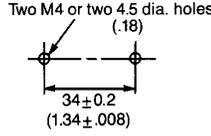
**Mounting dimensions of relay with socket**
