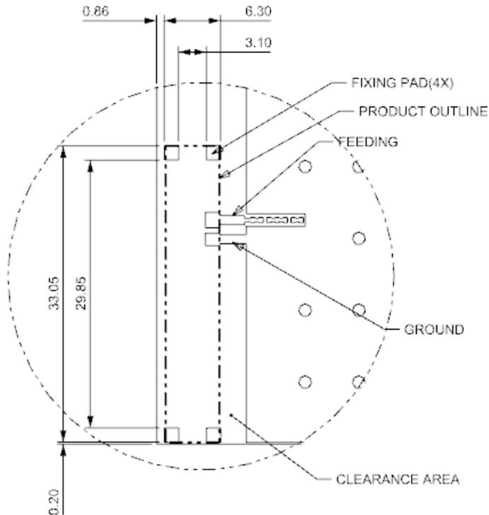
**FIGURE 7.5 RECOMMENDED FOOTPRINT ON PCB FOR SOLDERING**
