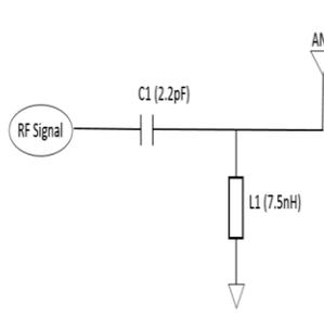
FIGURE 5.4 Matching Circuit for Reference Design
