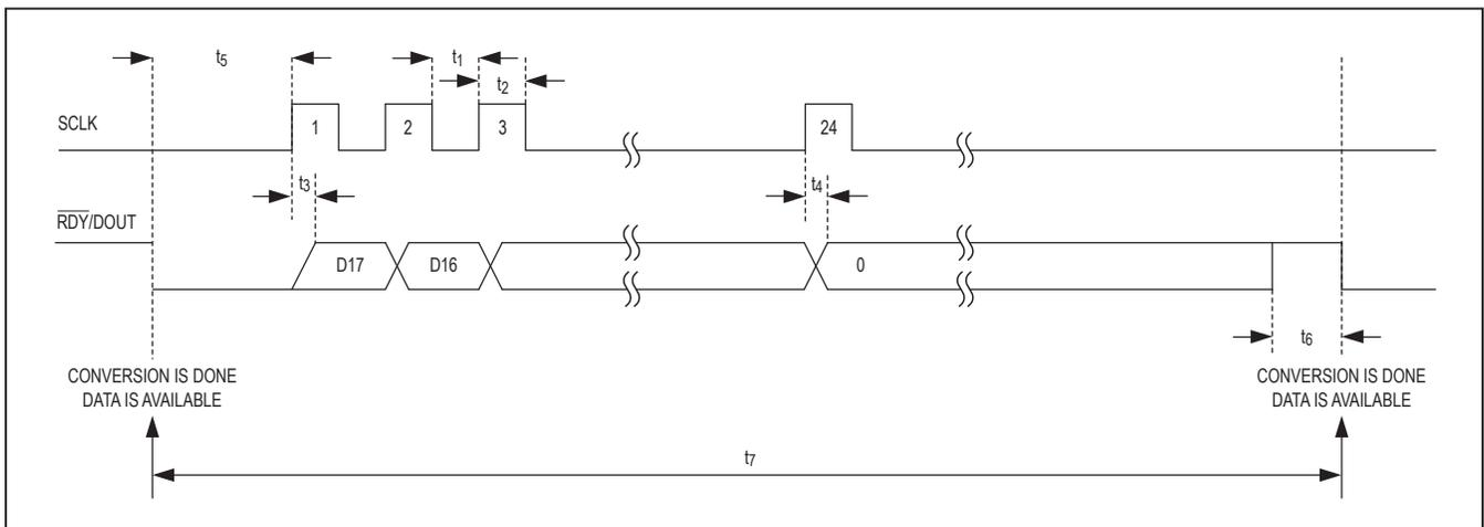
Figure 1. Timing Diagram for Data Read After Conversion
