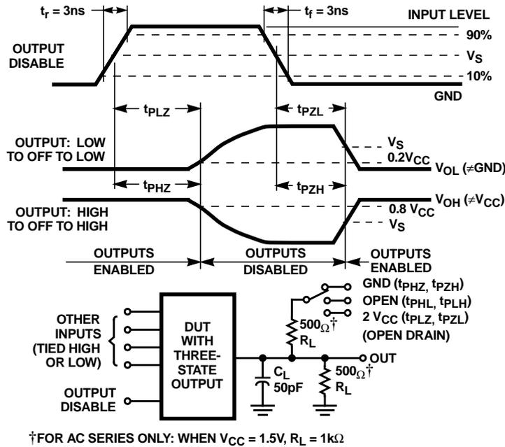
**FIGURE 1. THREE-STATE PROPAGATION DELAY TIMES AND TEST CIRCUIT**
