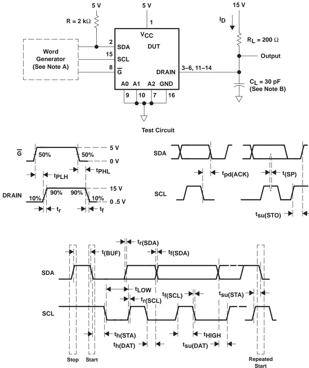
NOTES: A. The word generator has the following characteristics:  $t_r \leq 30$  ns,  $t_f \leq 30$  ns, pulsed repetition rate (PRR) = 400 kHz,  $Z_O = 50 \Omega$ .
