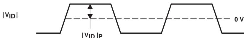
**Figure 5. Differential Input Voltage (Peak-to-Peak) Timing Waveform**
