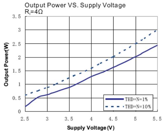
**Typical Performance Characteristics** (cont.) (@ $T_A = +25^\circ\text{C}$ , unless otherwise specified.)
