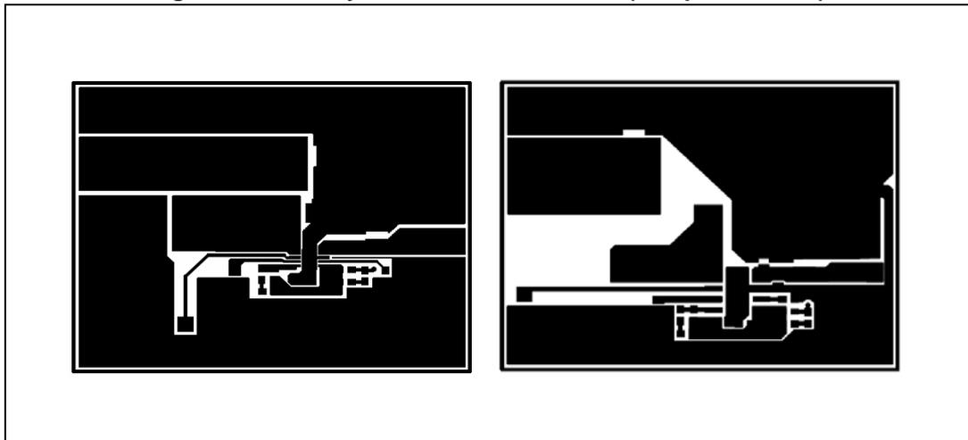
Figure 20. PCB layout: L7985 and L7985A (bottom side)
