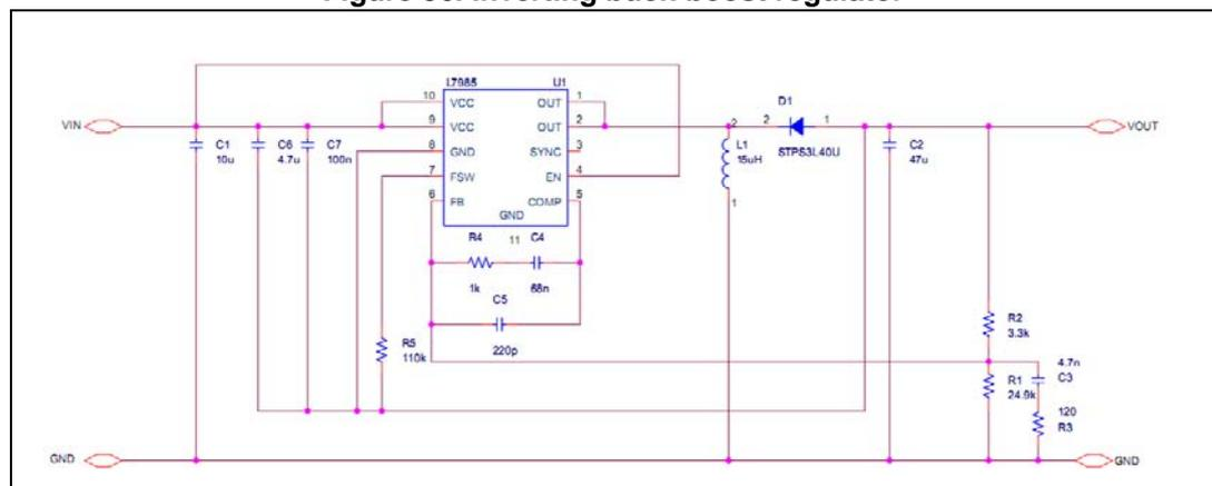
The GND pin of the device is connected to the output voltage so, given the output voltage, the input voltage range is limited by the maximum voltage the device can withstand across
