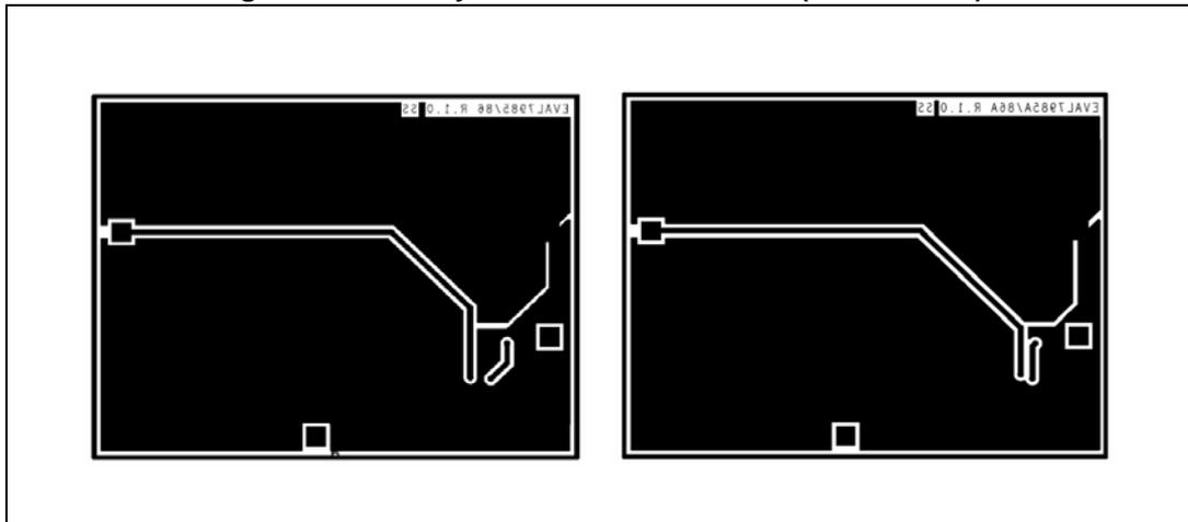
Figure 21. PCB layout: L7985 and L7985A (front side)
