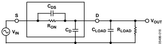
Figure 19. Switch Represented by Equivalent Parasitic Components
