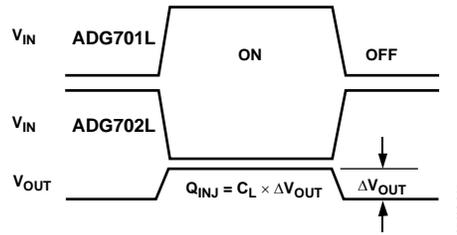
Figure 16. Charge Injection
