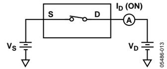
Figure 14. On Leakage
