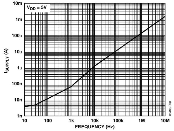
Figure 9. Supply Current vs. Input Switching Frequency
