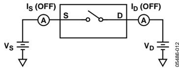
Figure 13. Off Leakage
