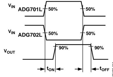
Figure 15. Switching Times
