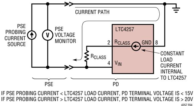
**Figure 4. IEEE 802.af Measured-Voltage Method of Classification Probing**
