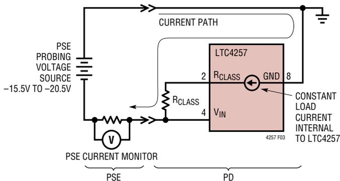
**Figure 3. IEEE 802.3af Measured-Current Method of Classification Probing**
