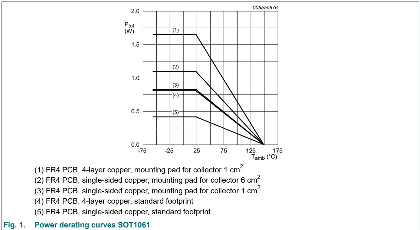
**Fig. 1. Power derating curves SOT1061**
