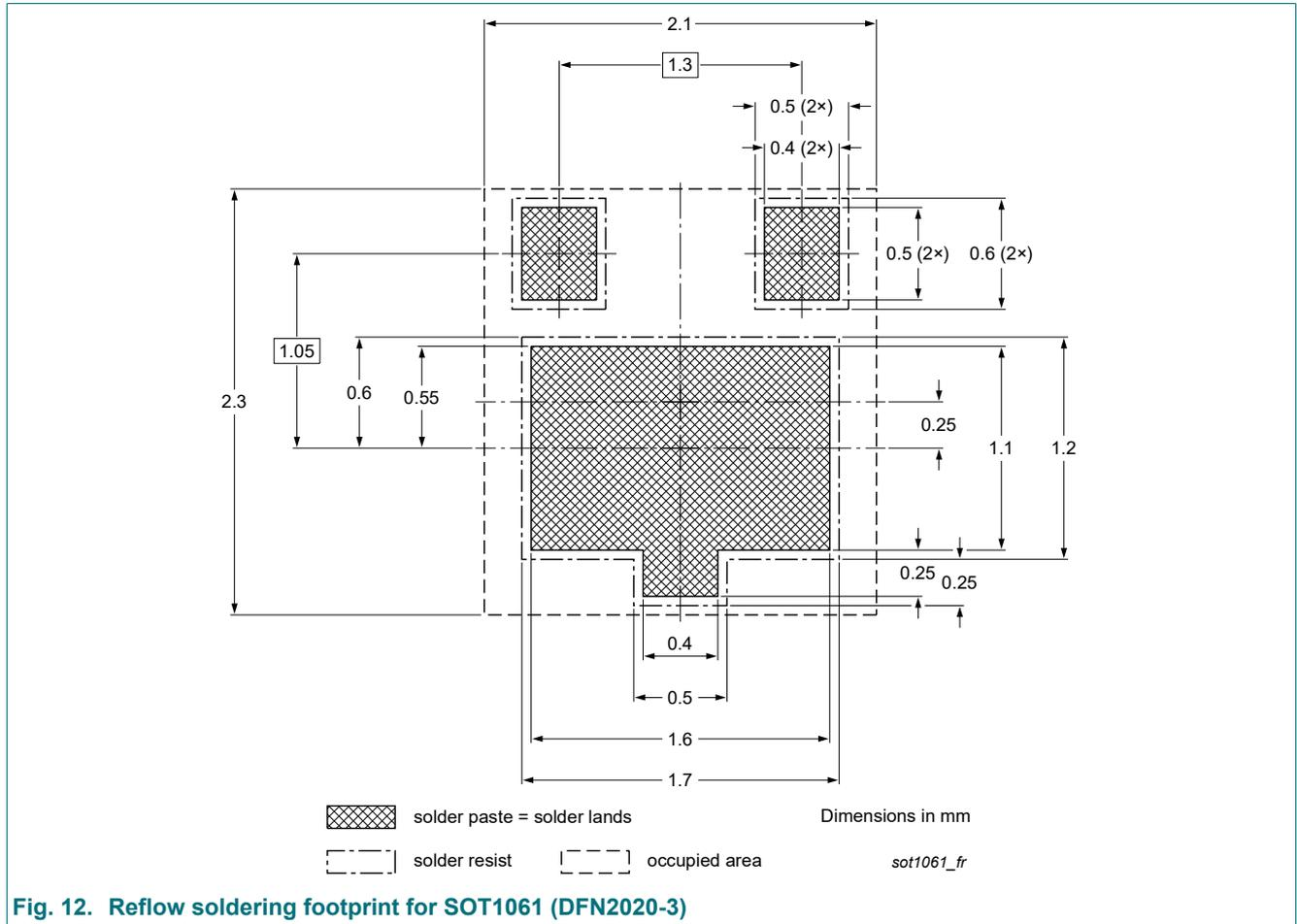
Fig. 12. Reflow soldering footprint for SOT1061 (DFN2020-3)
