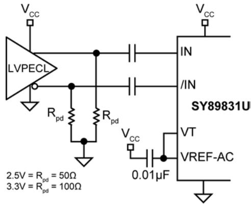
Figure 6. AC-Coupled LVPECL Input Interface
