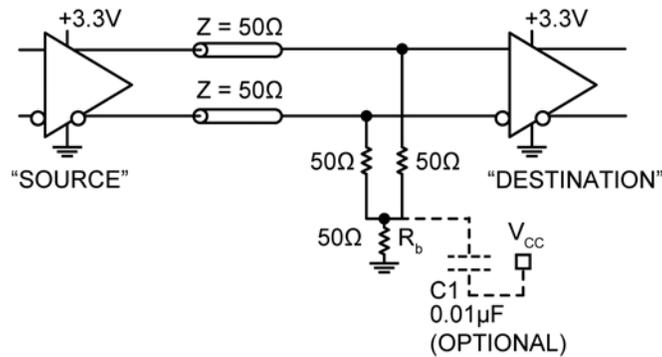
Figure 12. Three-Resistor ‘Y-Termination’
