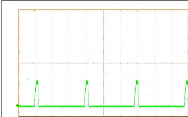
**Figure 8-18. Inductor Current Bursts During Hiccup**
