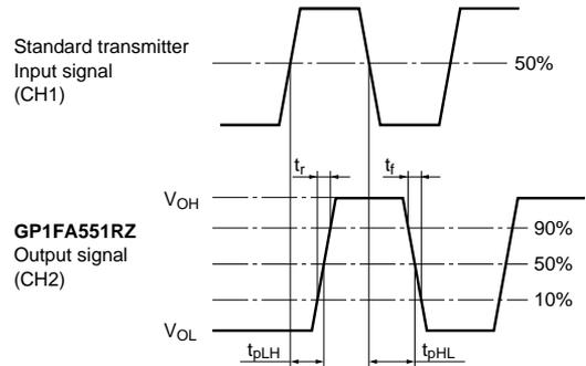
Fig.6 Measuring Method of Jitter
