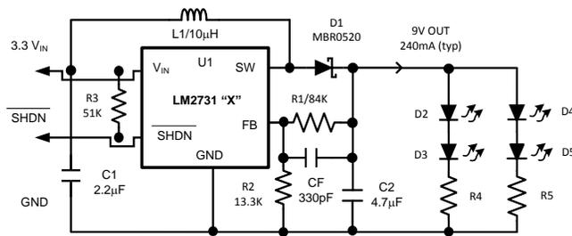
Figure 38. VIN = 3.3 V, VOUT = 9 V at 240 mA
