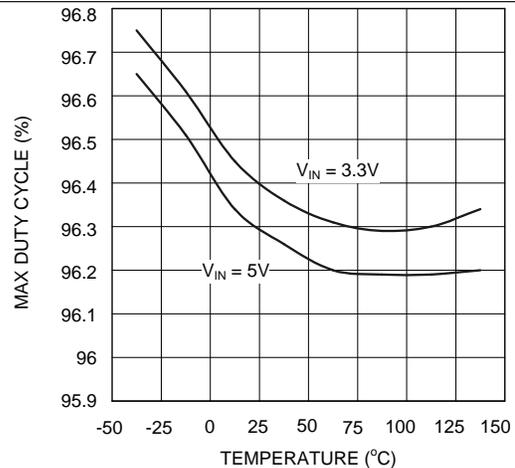
Figure 6. Maximum Duty Cycle vs Temperature - Y Option
