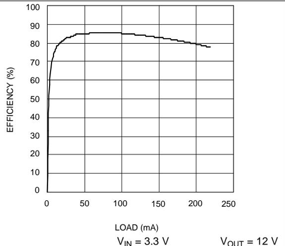
Figure 22. Efficiency vs Load Current - Y Option
