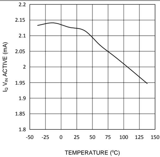
Figure 1.  $I_{q\ V_{IN}}$  (Active) vs Temperature - X Option
