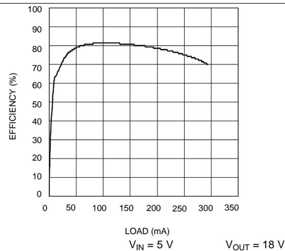
Figure 17. Efficiency vs Load Current - X Option
