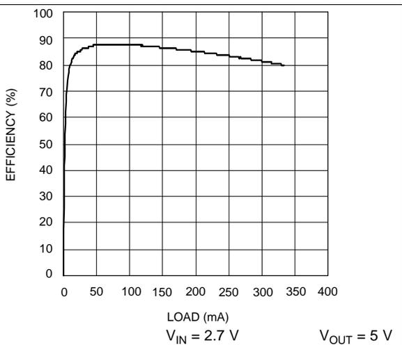
Figure 18. Efficiency vs Load Current - Y Option
