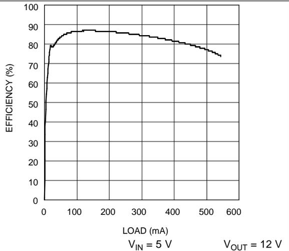
Figure 16. Efficiency vs Load Current - X Option
