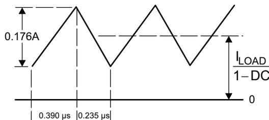
**Figure 27. 10 μH Inductor Current, 5 V–12 V Boost (LM2731X)**
