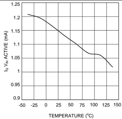
Figure 2.  $I_{q\ V_{IN}}$  (Active) vs Temperature - Y Option
