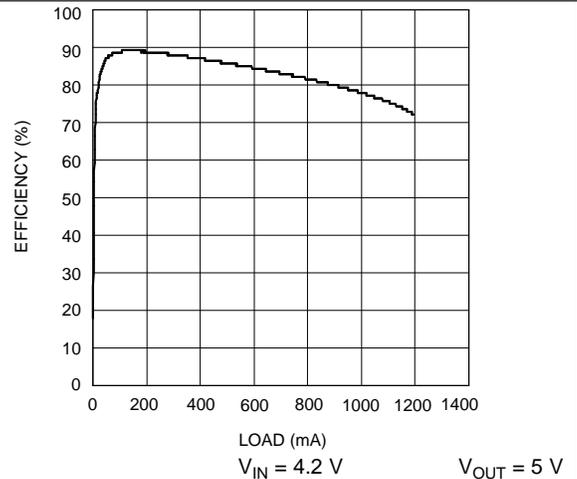
Figure 14. Efficiency vs Load Current - X Option
