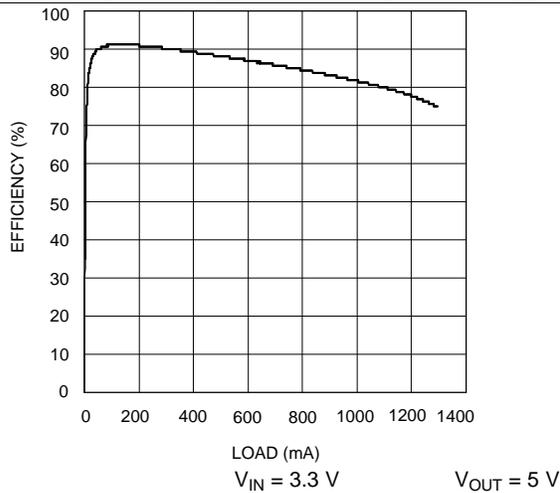
Figure 19. Efficiency vs Load Current - Y Option
