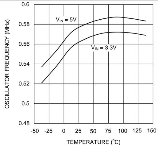
Figure 4. Oscillator Frequency vs Temperature - Y Option
