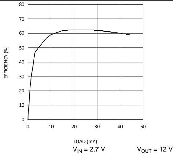
Figure 15. Efficiency vs Load Current - X Option
