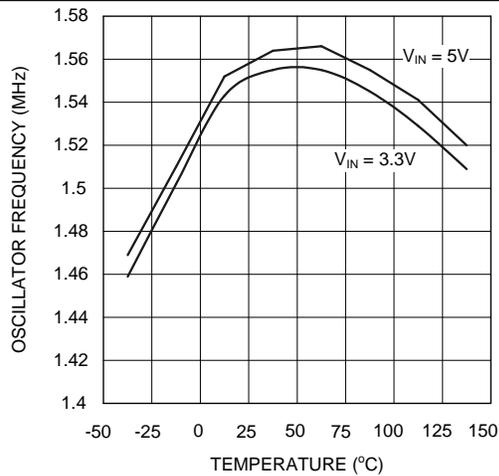
Figure 3. Oscillator Frequency vs Temperature - X Option
