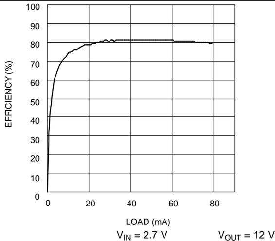
Figure 21. Efficiency vs Load Current - Y Option
