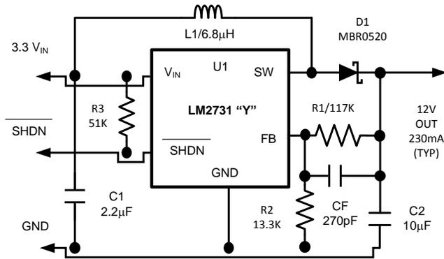
Figure 36. VIN = 3.3 V, VOUT = 12 V at 230 mA
