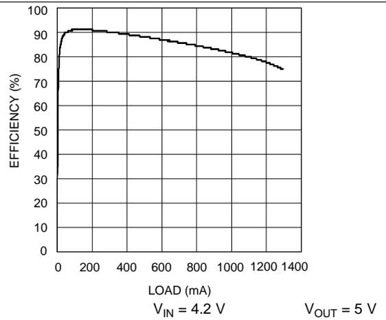
Figure 20. Efficiency vs Load Current - Y Option
