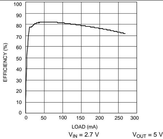
Figure 13. Efficiency vs Load Current - X Option
