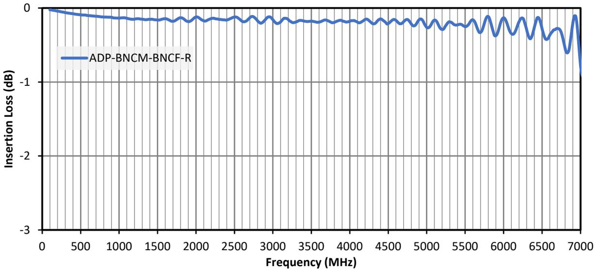
Figure 2. Insertion Loss for the ADP-BNCF-R Adapter
