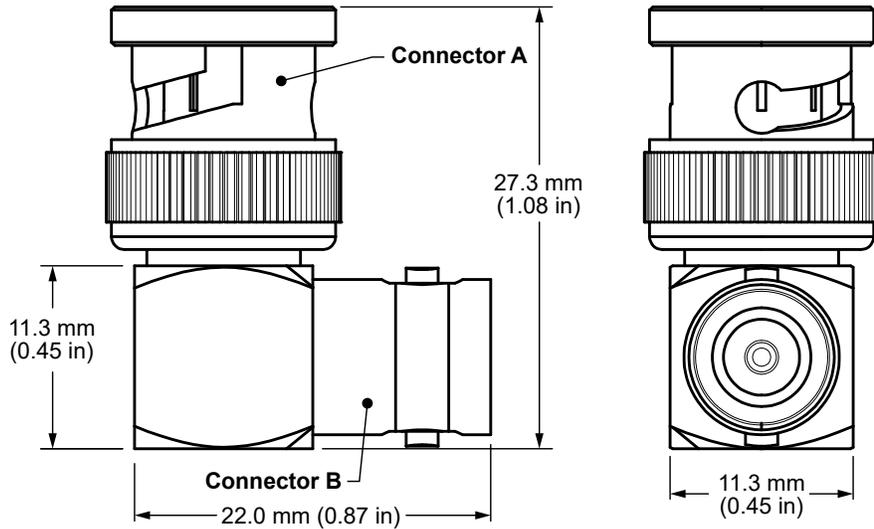
Figure 1. Product Dimensions for the ADP-BNCF-R Adapter
