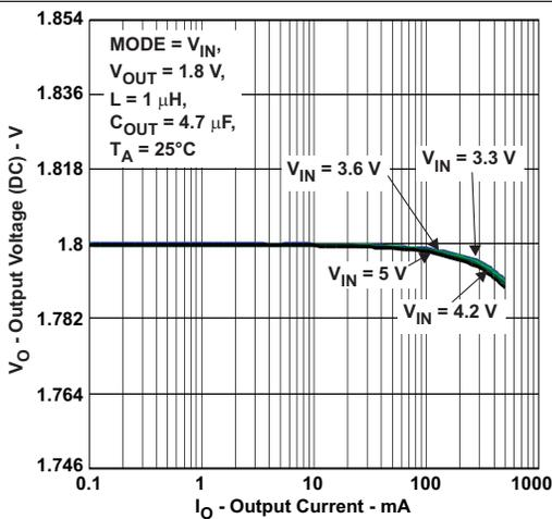
Figure 10. 1.8-V Output-Voltage Accuracy, Forced PWM Mode
