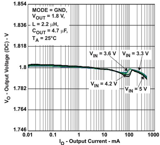
Figure 9. 1.8-V Output-Voltage Accuracy, PFM and PWM Mode
