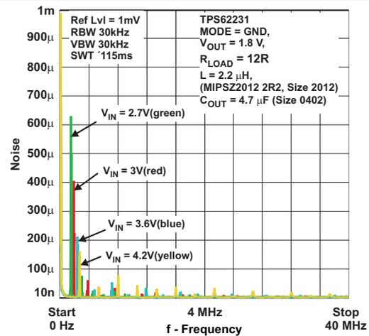
Figure 23. TPS62231-Q1: Spurious Output Noise, 12R Load
