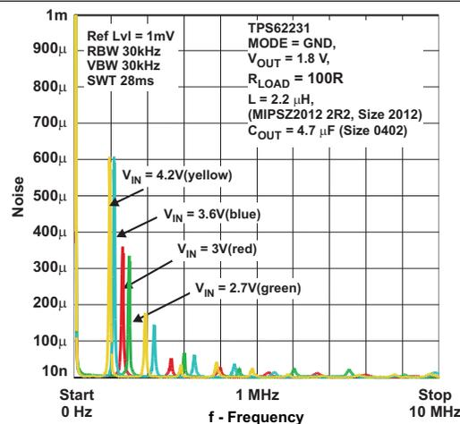
Figure 24. TPS62231-Q1: Spurious Output Noise, 100R Load
