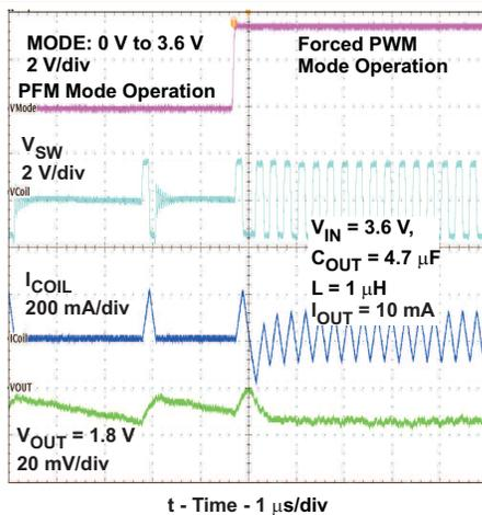
Figure 18. Mode Transition: PFM and Forced PWM Mode
