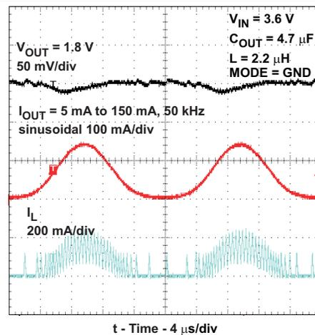
Figure 19. AC Load-Regulation Performance: 1.8-V  $V_{OUT}$ , PFM Mode
