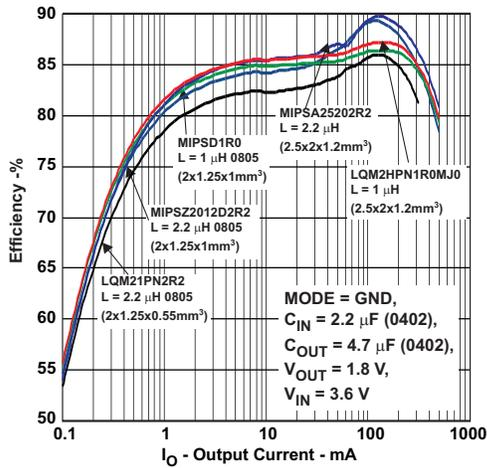
Figure 8. Comparison Efficiency vs Inductor Value and Size
