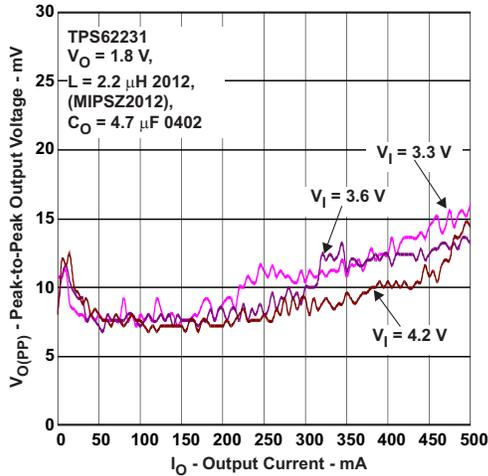
Figure 14. TPS62231-Q1: Output Voltage, Peak-to-Peak vs Output Current
