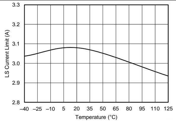
**Figure 26. Low-Side Current Limit vs Junction Temperature**
