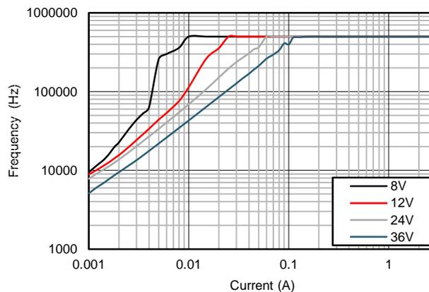
**Figure 45.  $V_{OUT} = 5\text{ V}$ ,  $F_s = 500\text{ kHz}$
