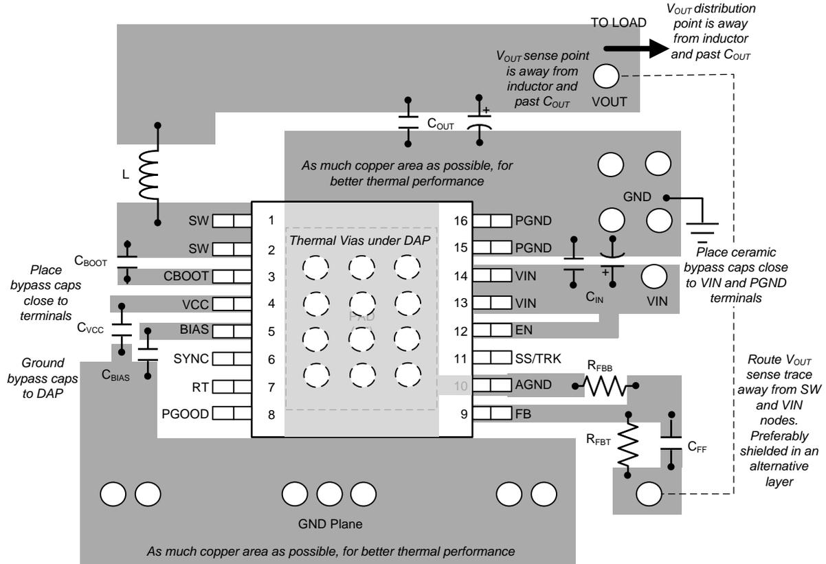
Figure 99. LM43603-Q1 Board Layout Recommendations
