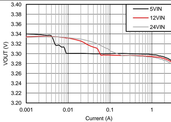
Figure 7.  $V_{OUT}$  Regulation
