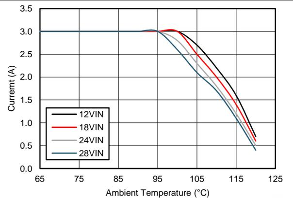
$V_{OUT} = 5\text{ V}$        $F_S = 500\text{ kHz}$        $R_{\theta JA} = 20^\circ\text{C/W}$
