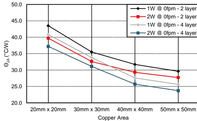
**Figure 98.  $R_{\theta JA}$  vs Copper Area**
