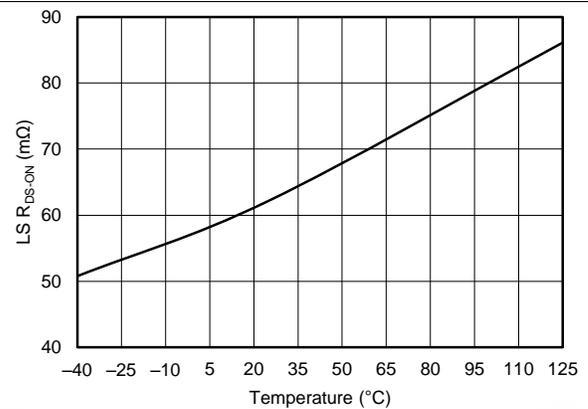
**Figure 24. Low-Side FET On Resistance vs Junction Temperature**
