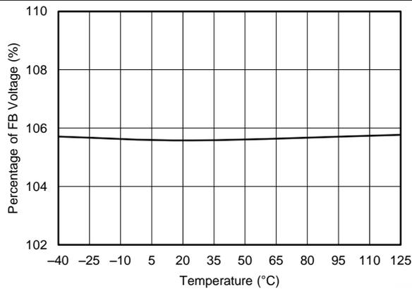
**Figure 27. PGOOD OVP Falling Threshold vs Junction Temperature**
