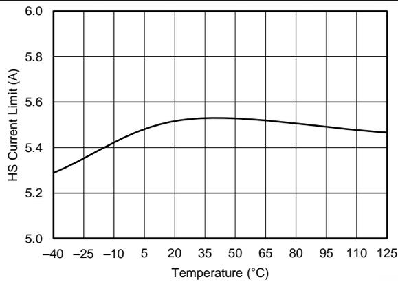
**Figure 25. High-Side Current Limit vs Junction Temperature**
