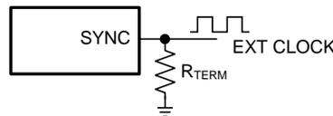
**Figure 42. Frequency Synchronization**
