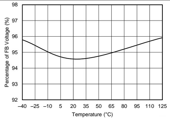
**Figure 30. PGOOD UVP Rising Threshold vs Junction Temperature**
