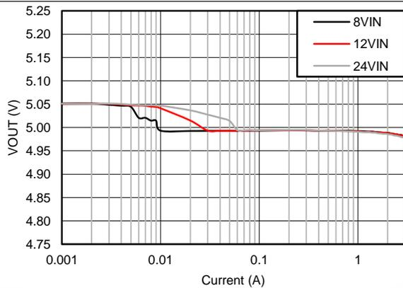
Figure 9.  $V_{OUT}$  Regulation
