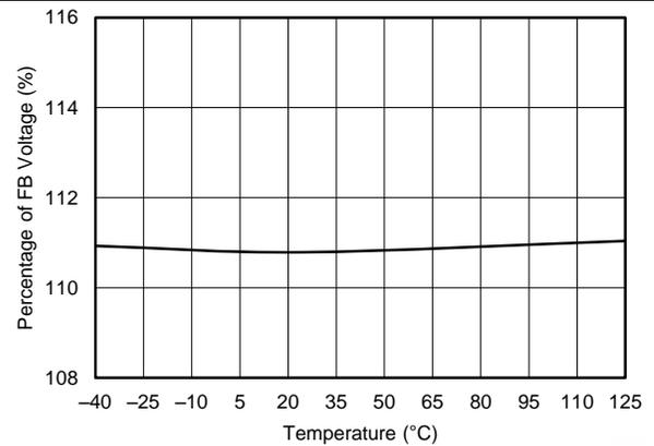
**Figure 28. PGOOD OVP Rising Threshold vs Junction Temperature**
