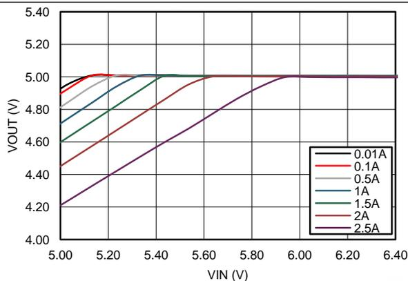
$V_{OUT} = 5\text{ V}$   $F_S = 2.2\text{ MHz}$
