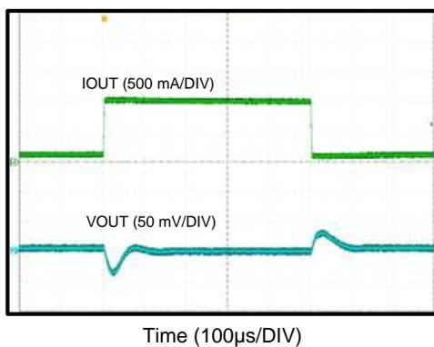
$V_{IN} = 12\text{ V}$        $V_{OUT} = 1\text{ V}$
