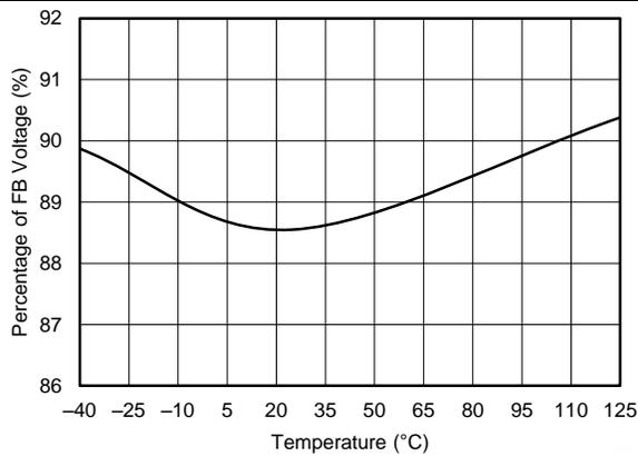
**Figure 29. PGOOD UVP Falling Threshold vs Junction Temperature**
