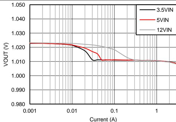
$V_{OUT} = 1\text{ V}$        $F_S = 500\text{ kHz}$
