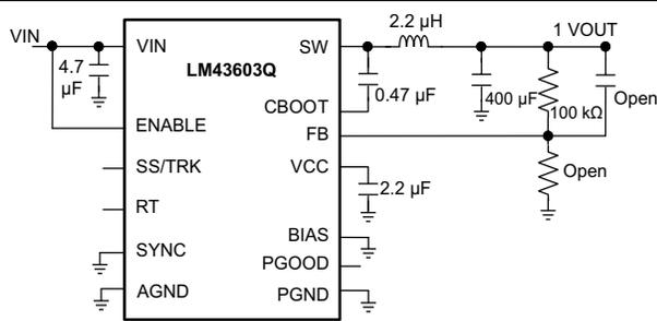
$V_{OUT} = 1\text{ V}$        $F_S = 500\text{ kHz}$
