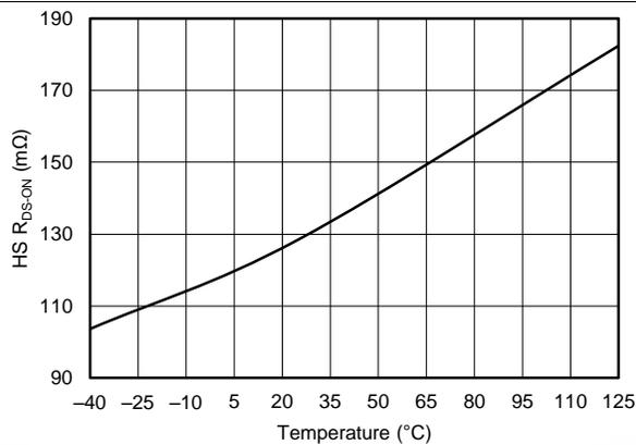
**Figure 23. High-Side FET On Resistance vs Junction Temperature**
