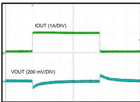
$V_{OUT} = 5\text{ V}$        $F_S = 500\text{ kHz}$
