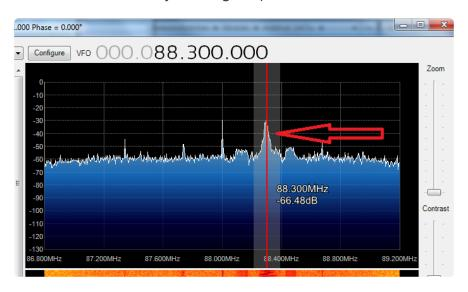
With the latest versions of SDR-Sharp it will automatically detect and decode RBDS/RDS data that is sent along with FM radio
