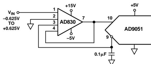
Figure 6. Level-Shifting with the AD830
