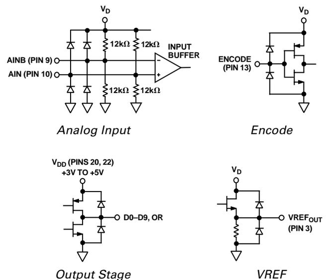
Figure 2. Equivalent Circuits
