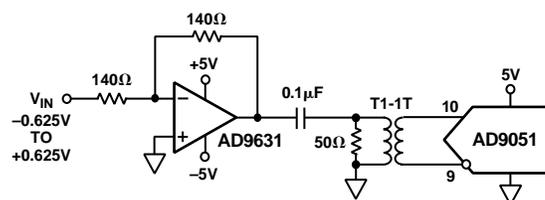
Figure 5. Differentially Driven AD9051 Using Transformer Coupling
