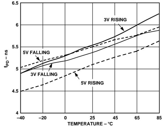
TPC 16.  $t_{PD}$  vs. Temperature 3 V/5 V
