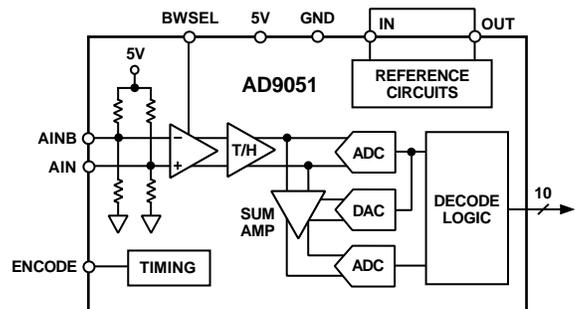
A 2.5 V reference is included onboard, or the user can provide an external reference voltage for gain control or matching of multiple devices. Fabricated on a state-of-the-art BiCMOS process, the AD9051 is packaged in a space saving surface mount package (SSOP) and is specified over the industrial temperature range ( $-40^{\circ}\text{C}$  to  $+85^{\circ}\text{C}$ ).
