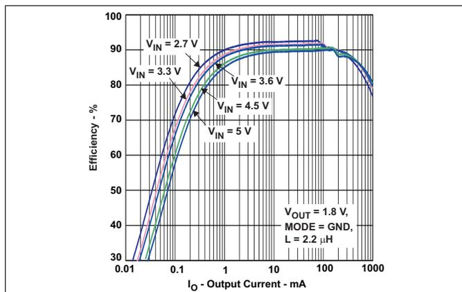
Figure 8. Efficiency (Power Save Mode) vs Output Current
