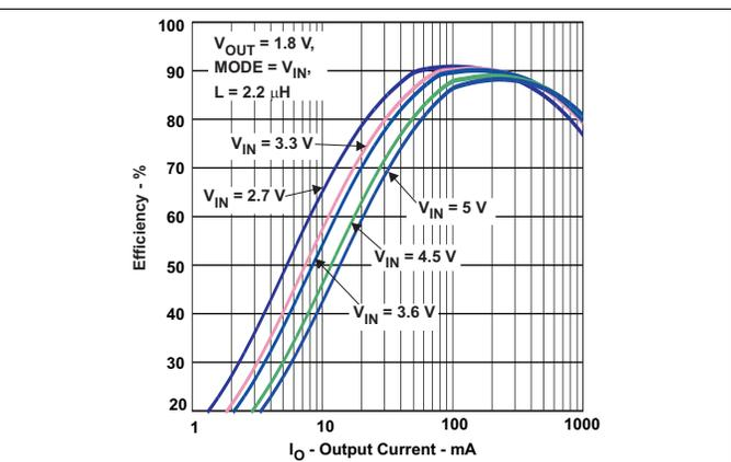
Figure 9. Efficiency (Forced PWM Mode) vs Output Current
