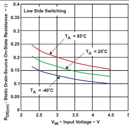
Figure 4. Static Drain-Source ON-State Resistance vs Input Voltage
