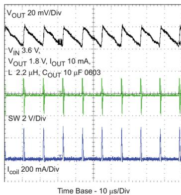
Figure 16. Typical Operation vs PFM Mode
