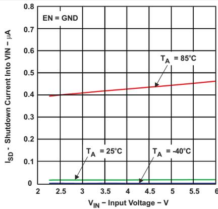
Figure 1. Shutdown Current into VIN vs Input Voltage
