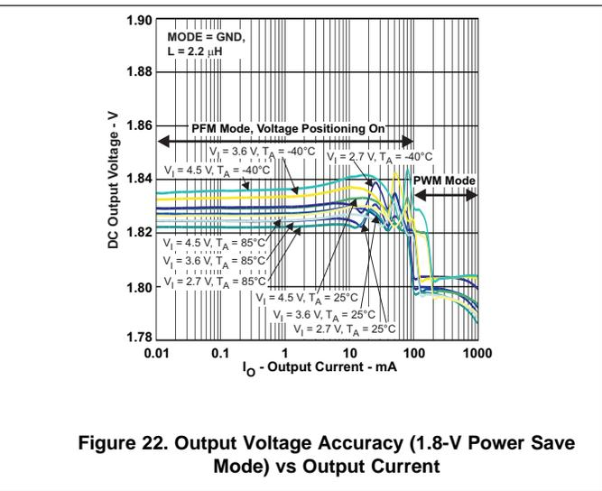
Figure 22. Output Voltage Accuracy (1.8-V Power Save Mode) vs Output Current
