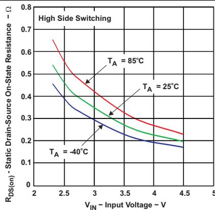
Figure 3. Static Drain-Source ON-State Resistance vs Input Voltage
