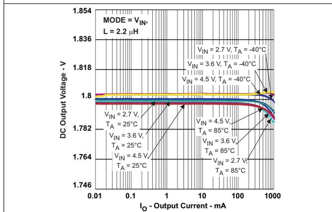
Figure 10. Output Voltage Accuracy (1.8-V Forced PWM Mode) vs Output Current
