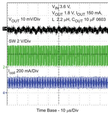
Figure 17. Typical Operation vs PWM Mode
