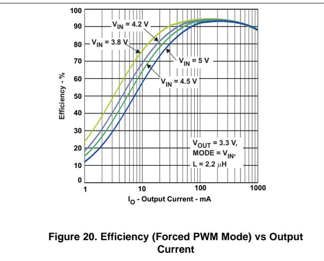
Figure 20. Efficiency (Forced PWM Mode) vs Output Current
