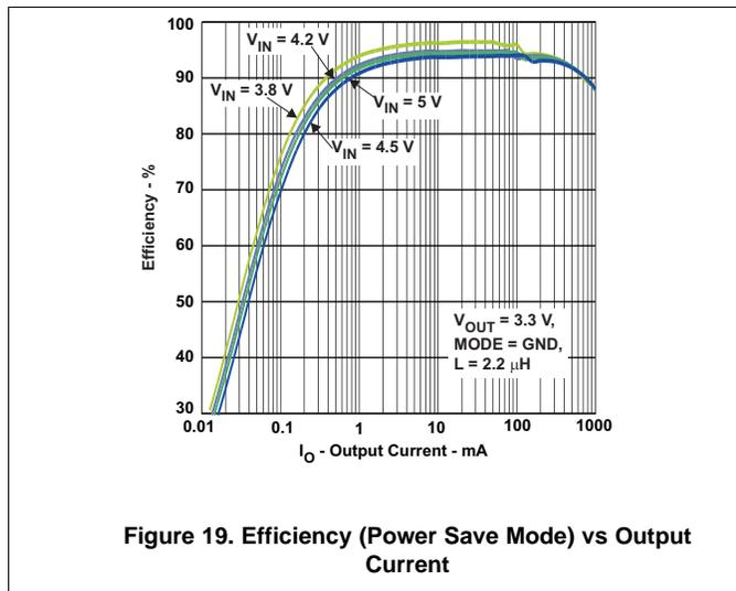
Figure 19. Efficiency (Power Save Mode) vs Output Current
