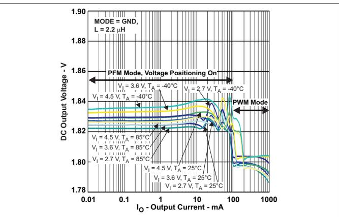
Figure 11. Output Voltage Accuracy (1.8-V Power Save Mode) vs Output Current
