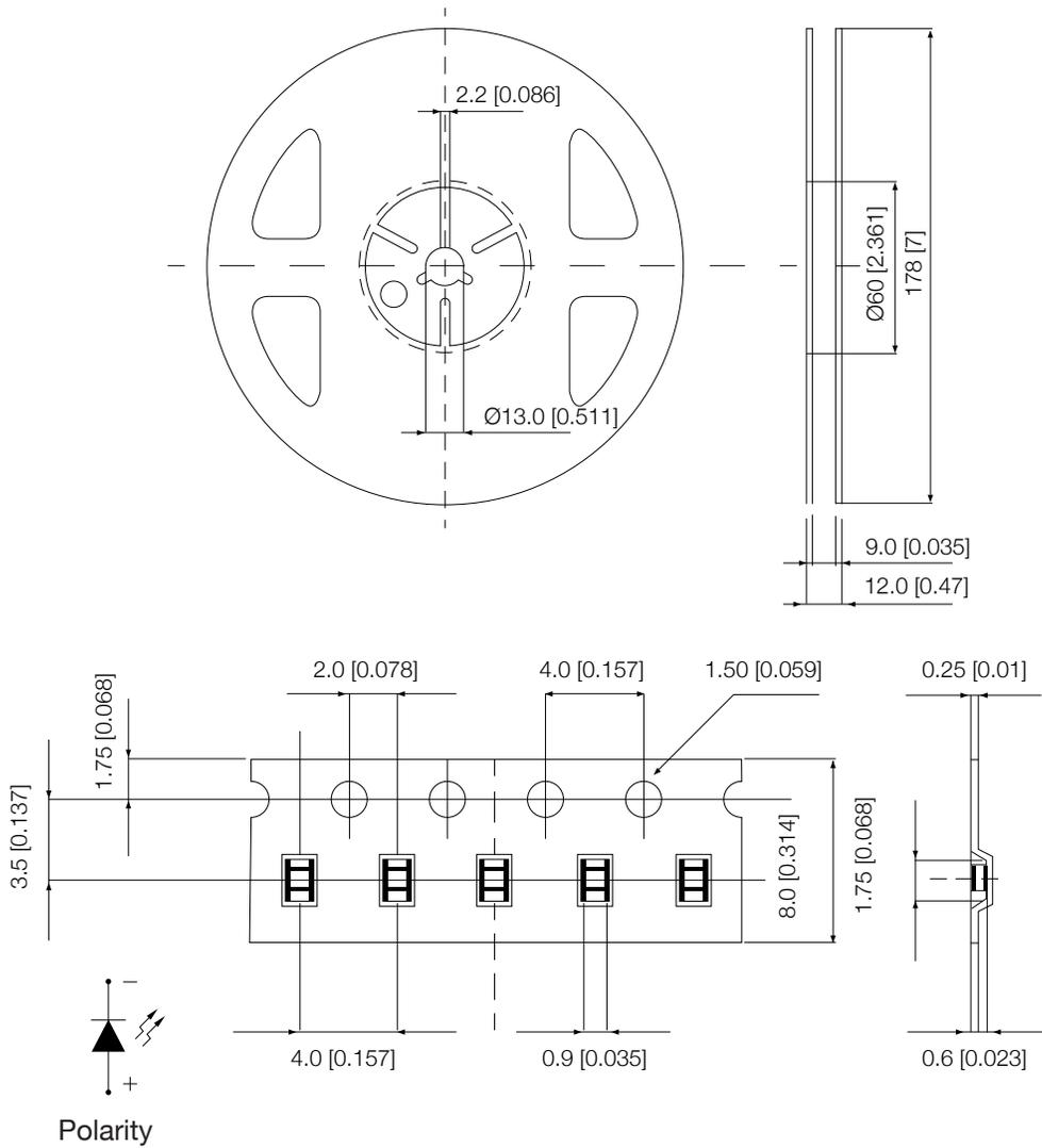
**Note:** The tolerance unless mentioned is  $\pm 0.1\text{mm}$  [0.005 in] ; Unit=mm [in]
