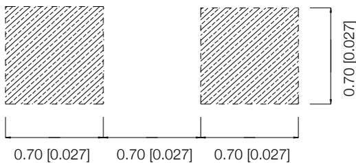
**Note:** The tolerance unless mentioned is  $\pm 0.1\text{mm}$  [0.005 in] ; Unit=mm [in]
