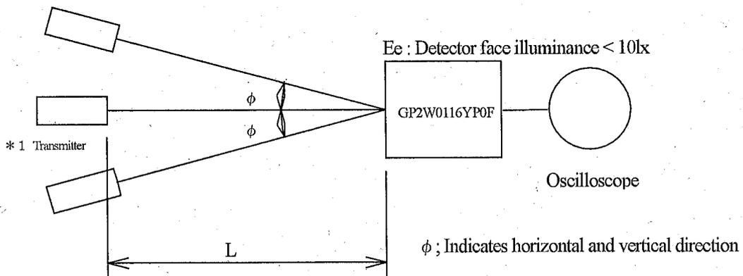
\*1 Transmitter shall use GP2W0116YP0F ( $\lambda_p=870nm$  TYP) which is adjusted the radiation intensity at 3.6mW/sr.
