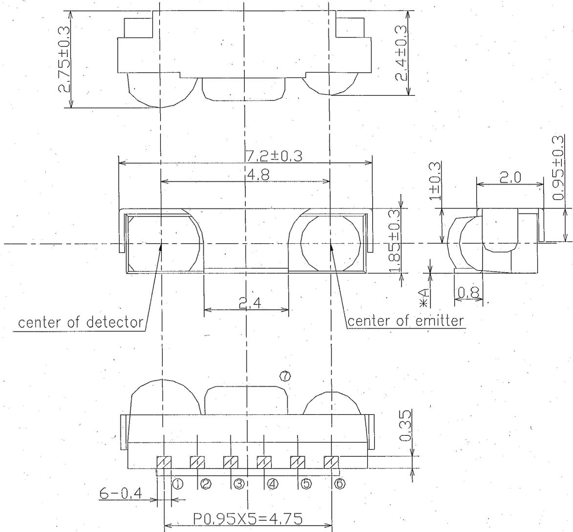
\*A : Distance between PCB of the transceiver and bottom side of the shield case shall be less than 0.1mm for both up and downward direction.
