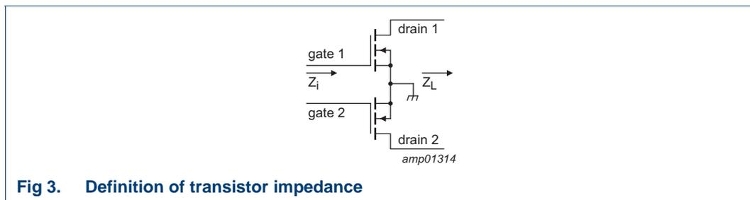
Fig 3. Definition of transistor impedance
