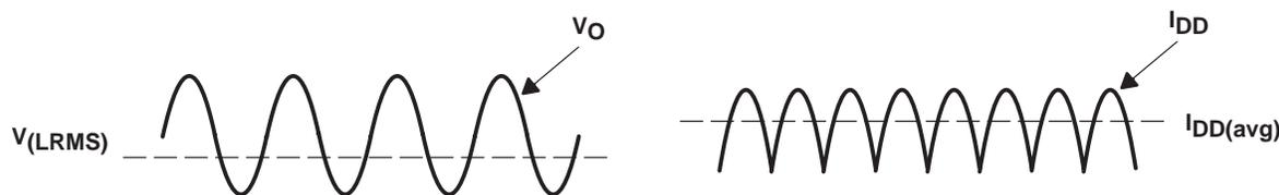
**Figure 26. Voltage and Current Waveforms for BTL Amplifiers**
