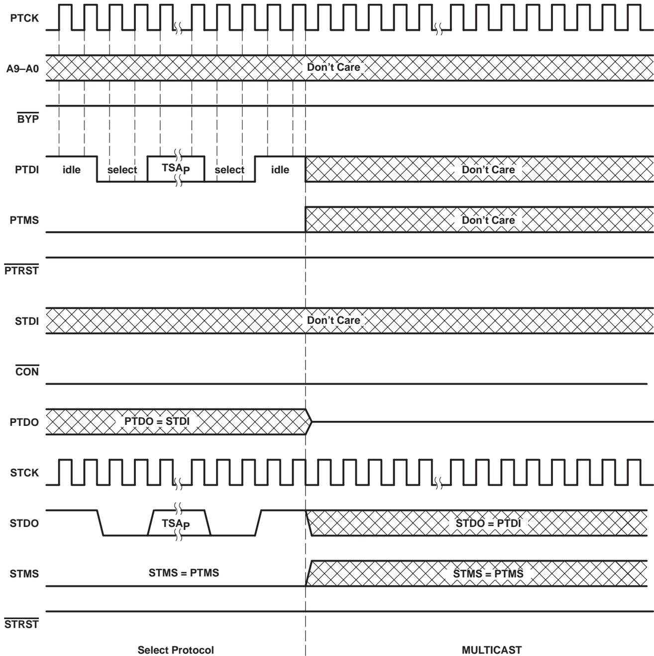
Figure 14. Shadow-Protocol Timing,
