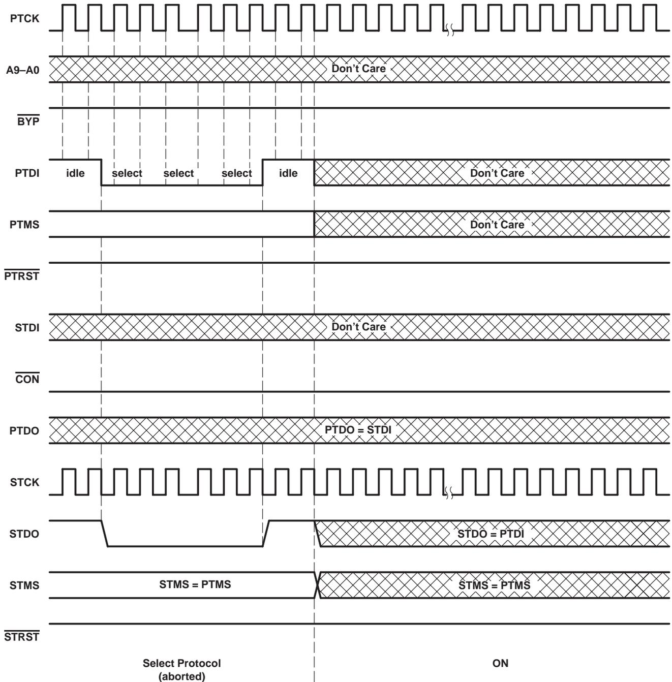
NOTE A: The sequence of PTDI bits shown in this figure is only one of many that would produce protocol result SOFT ERROR.
