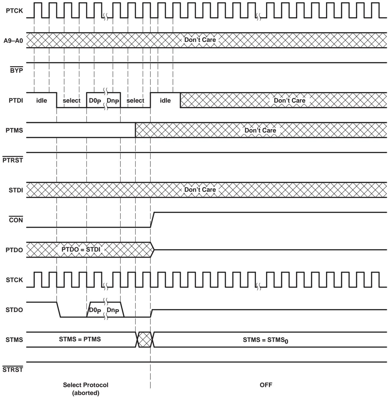
NOTE A: The position of PTMS shown in this figure is only one of many that would produce protocol result HARD ERROR.
