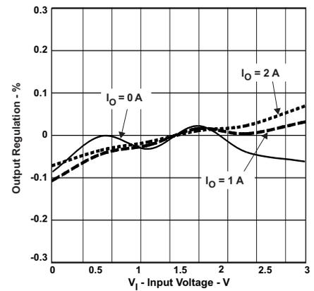
Figure 16. Input Regulation % vs. Input Voltage
