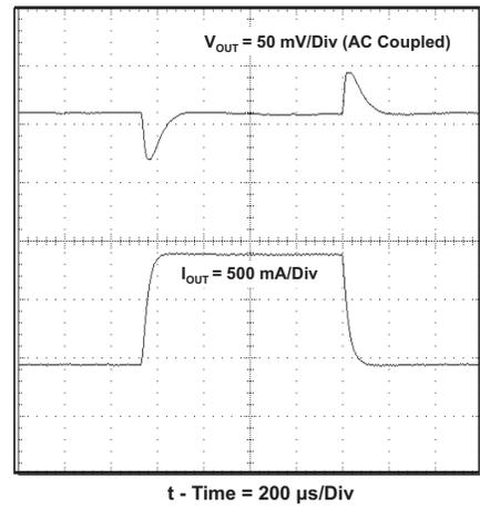
Figure 19. Transient Response,  $I_O$  Step 0.5 to 1.5 A
