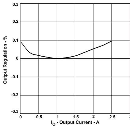
Figure 15. Output Regulation % vs. Output Current
