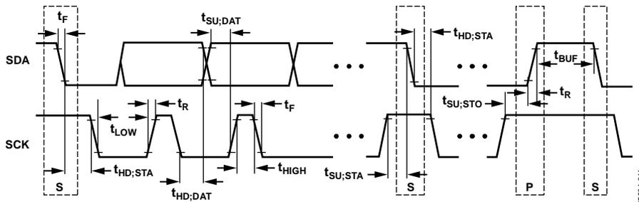
Figure 11. I<sup>2</sup>C Port Timing Diagram
