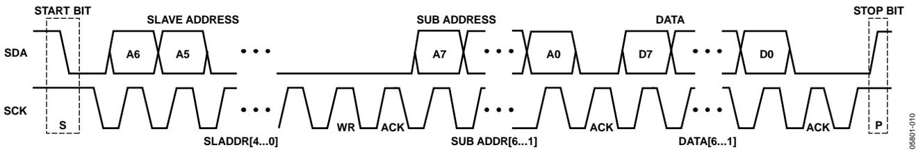
Figure 10. I<sup>2</sup>C Data Transfer Timing
