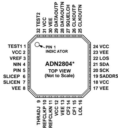
\*THERE IS AN EXPOSED PAD ON THE BOTTOM OF THE PACKAGE THAT MUST BE CONNECTED TO GND.
