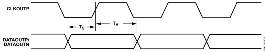
Figure 2. Output Timing
