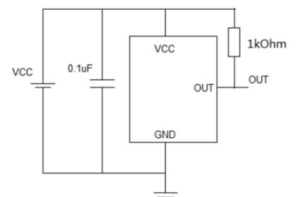
It is strongly recommended that an external bypass capacitor be connected in close proximity to the device between the supply and ground pins to reduce noise. The recommended value for the external bypass capacitor is 0.1µF.
