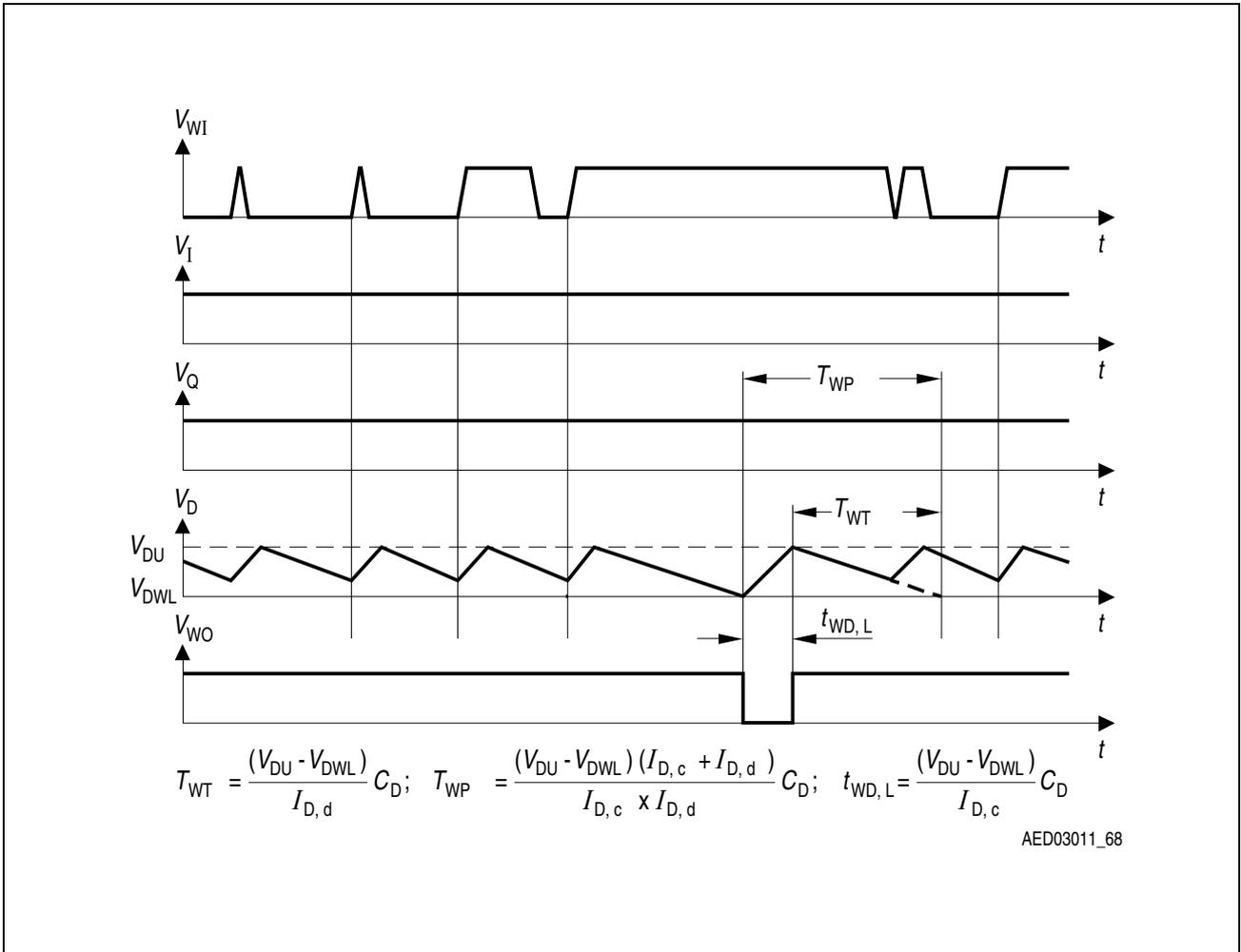
**Figure 6** Timing of the Watchdog Function
