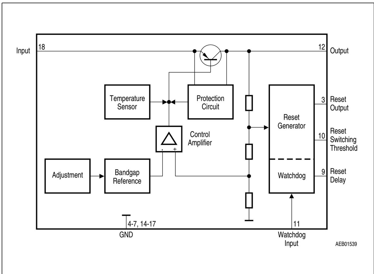
**Figure 3** Block Diagram TLE 4268 G (PG-DSO-20-35)
