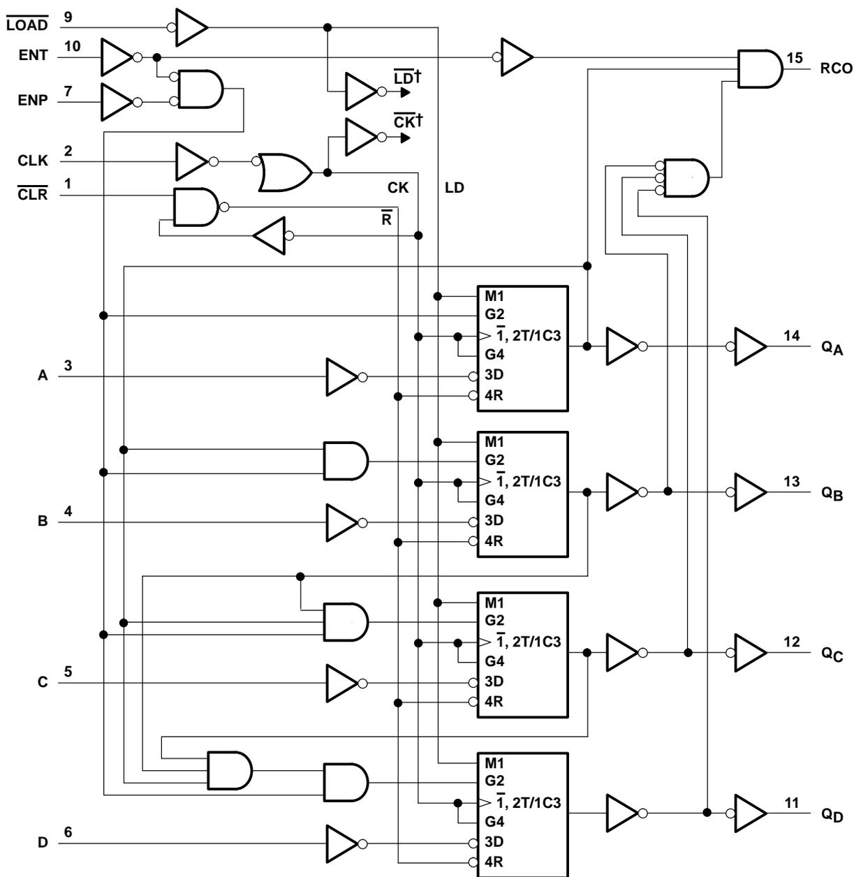
† For simplicity, routing of complementary signals  $\overline{LD}$  and  $\overline{CK}$  is not shown on this overall logic diagram. The uses of these signals are shown on the logic diagram of the D/T flip-flops.
