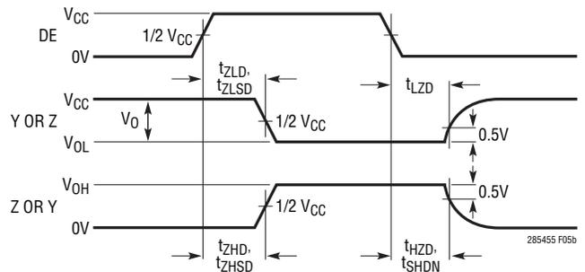
Figure 5. Driver Enable and Disable Timing Measurements
