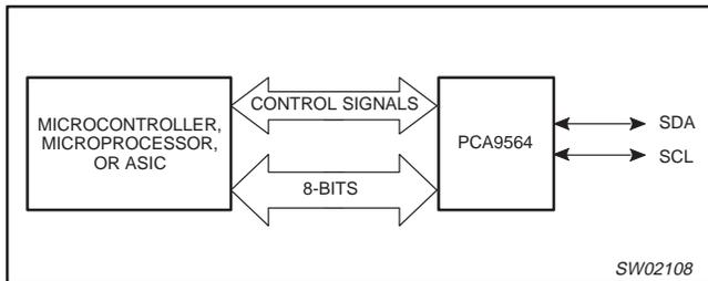
Figure 14. Adding I<sup>2</sup>C-bus Port Application
