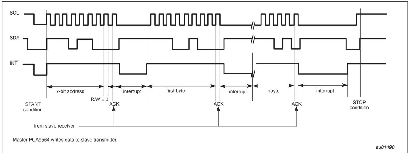
Figure 9. Bus timing diagram; master transmitter mode
