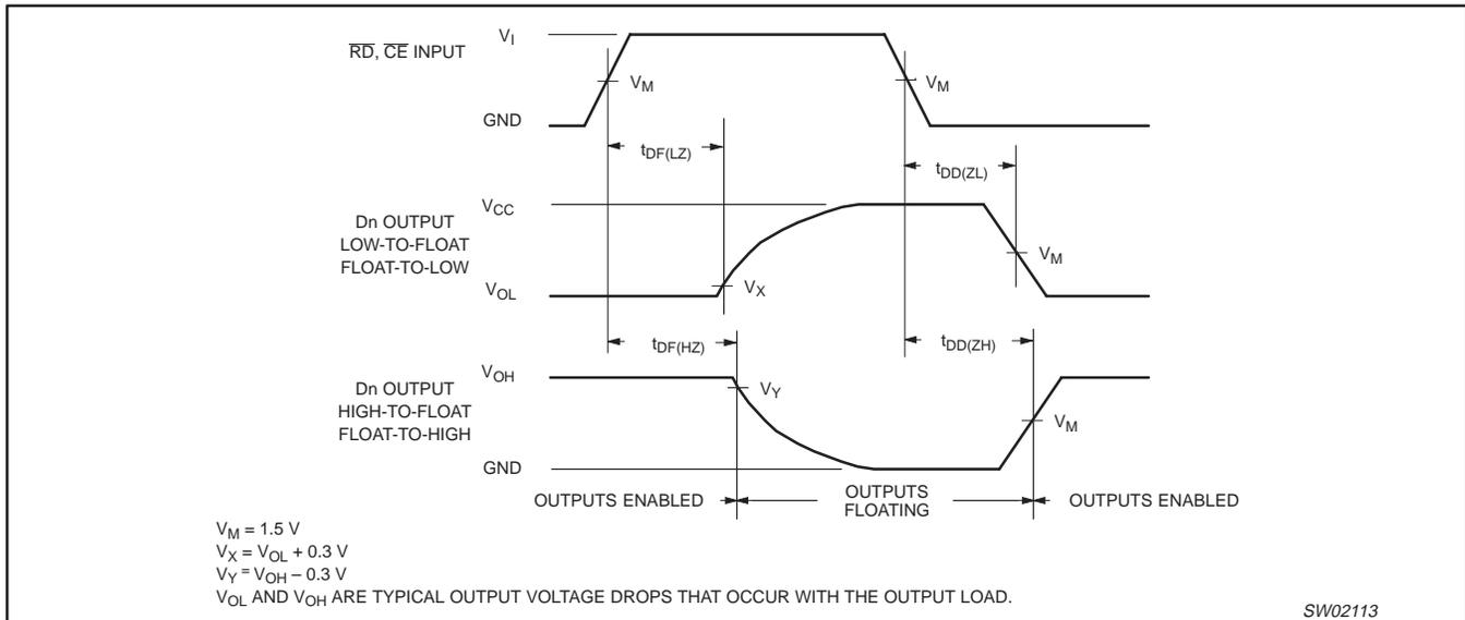
Figure 21. t<sub>DD</sub> and t<sub>DF</sub> times
