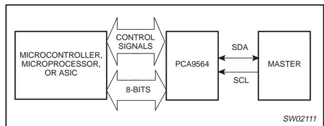
Figure 17. Converting Parallel to Serial Data Application
