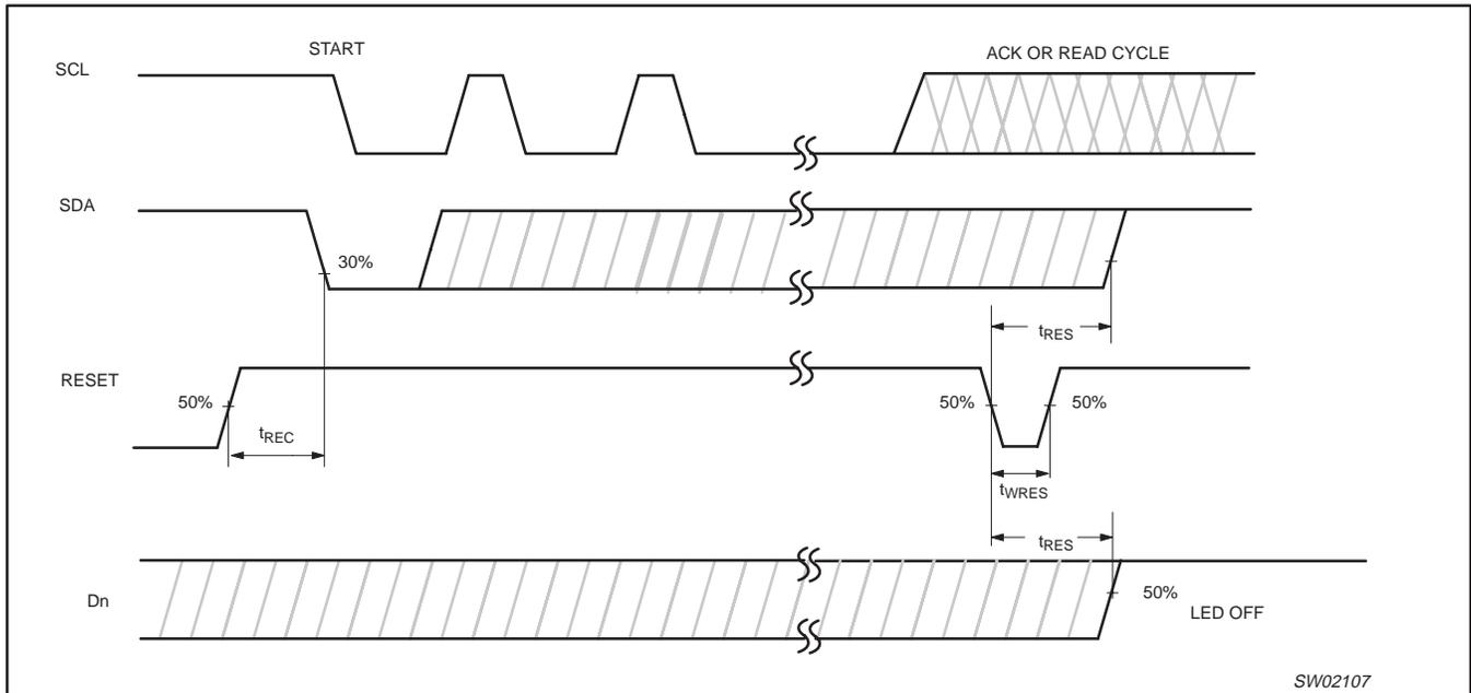
Figure 19. Reset timing
