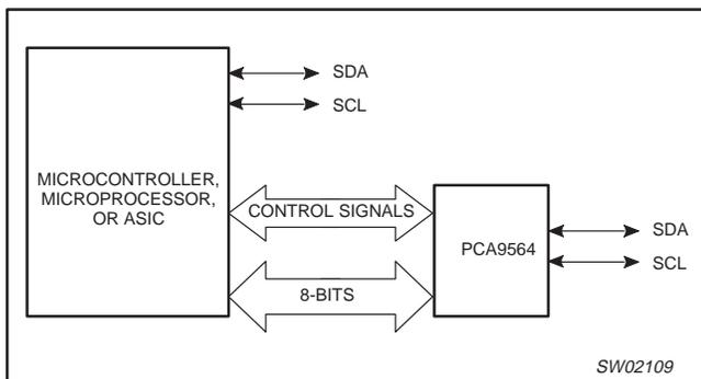
Figure 15. Adding Additional I<sup>2</sup>C-bus Ports Application
