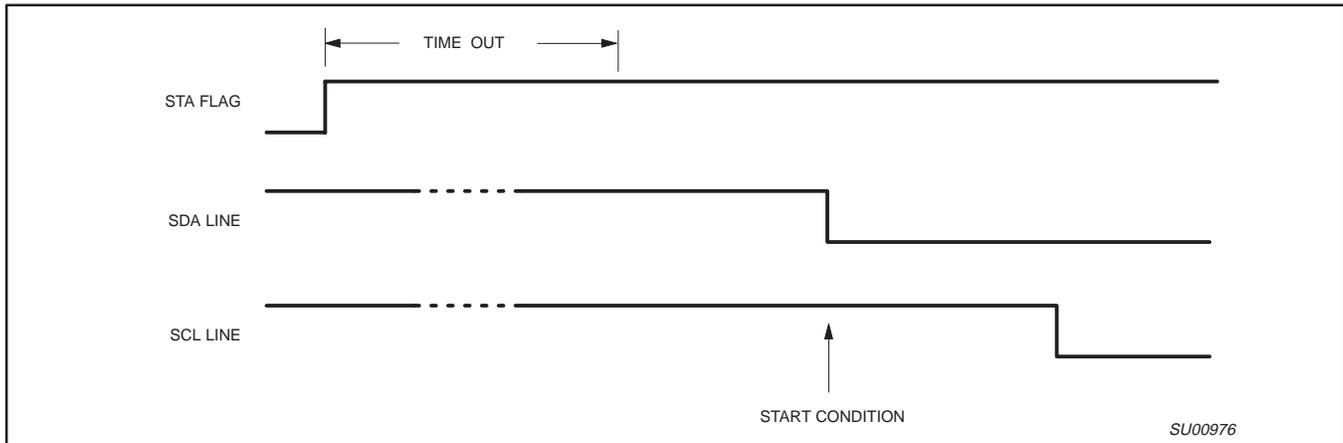
**Figure 7. Forced access to a busy I<sup>2</sup>C-bus**
