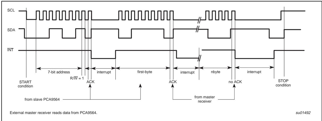
Figure 11. Bus timing diagram; slave transmitter mode
