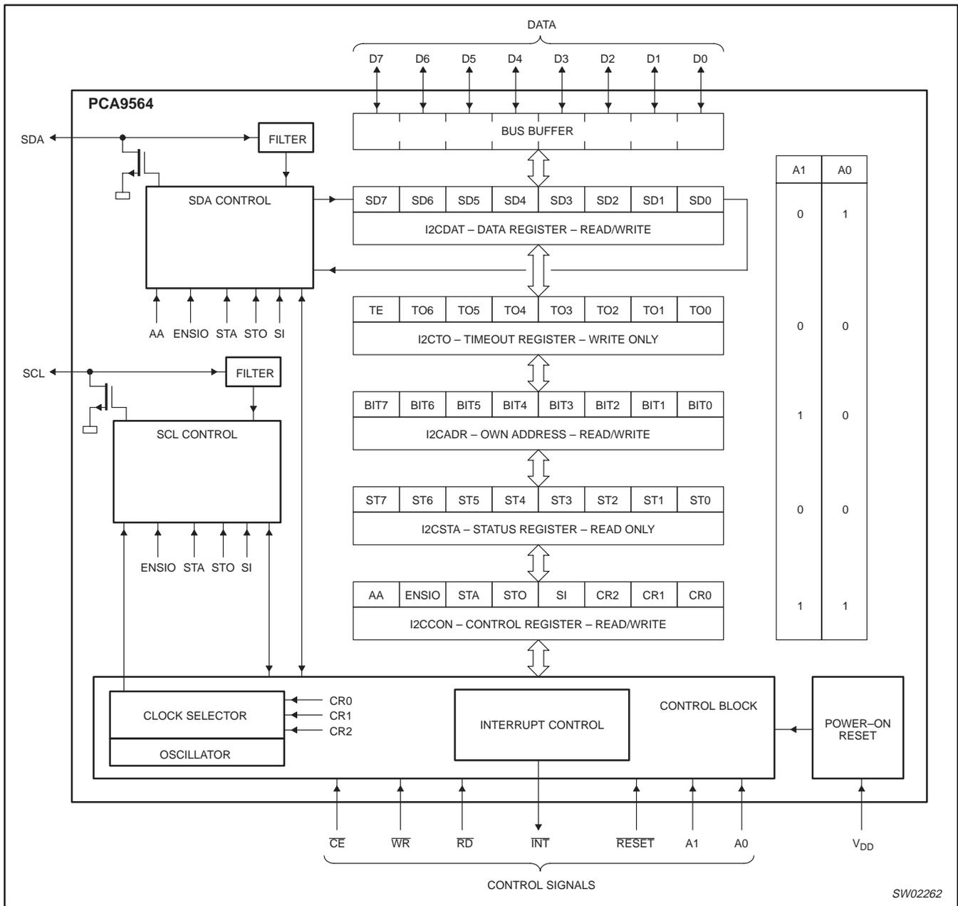
Figure 1. Block diagram
