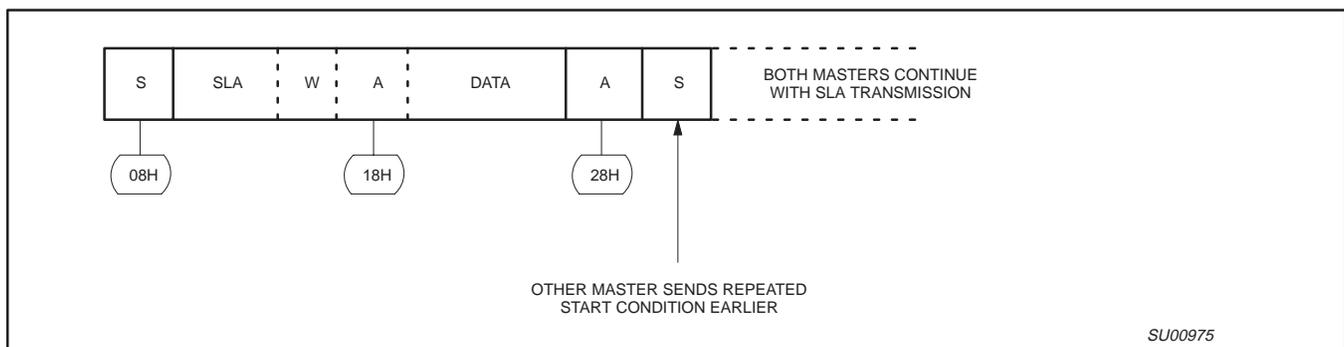
Figure 6. Simultaneous repeated START conditions from 2 masters
