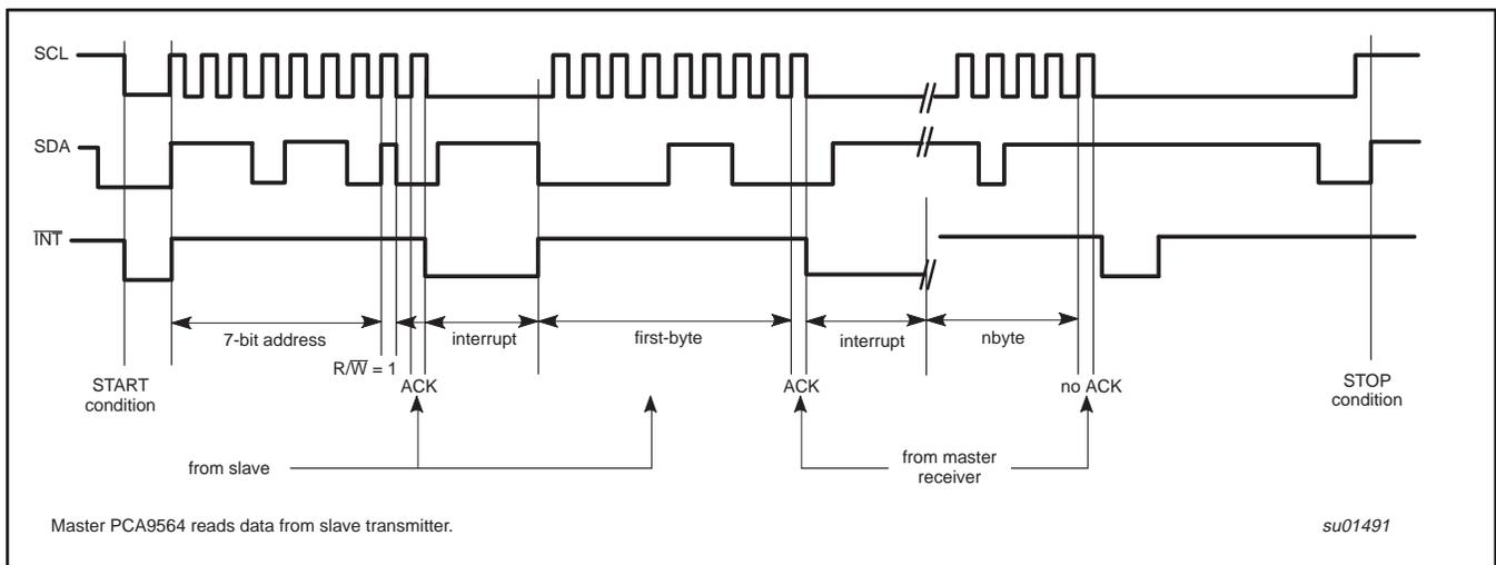
Figure 10. Bus timing diagram; master receiver mode
