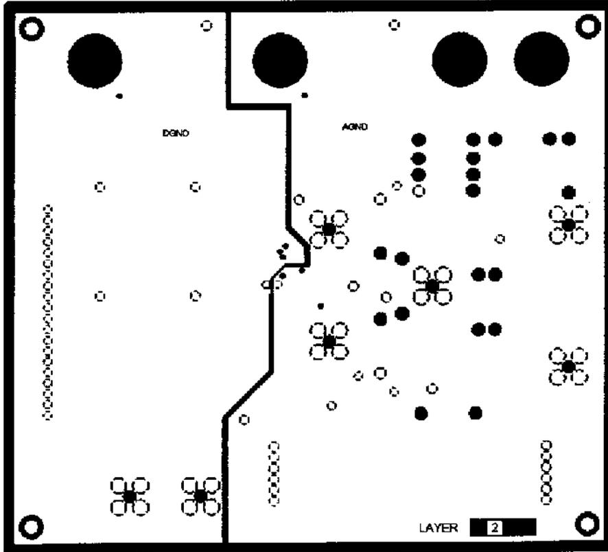
Figure 29. Ground Plane PCB Layout (Layer 2)
