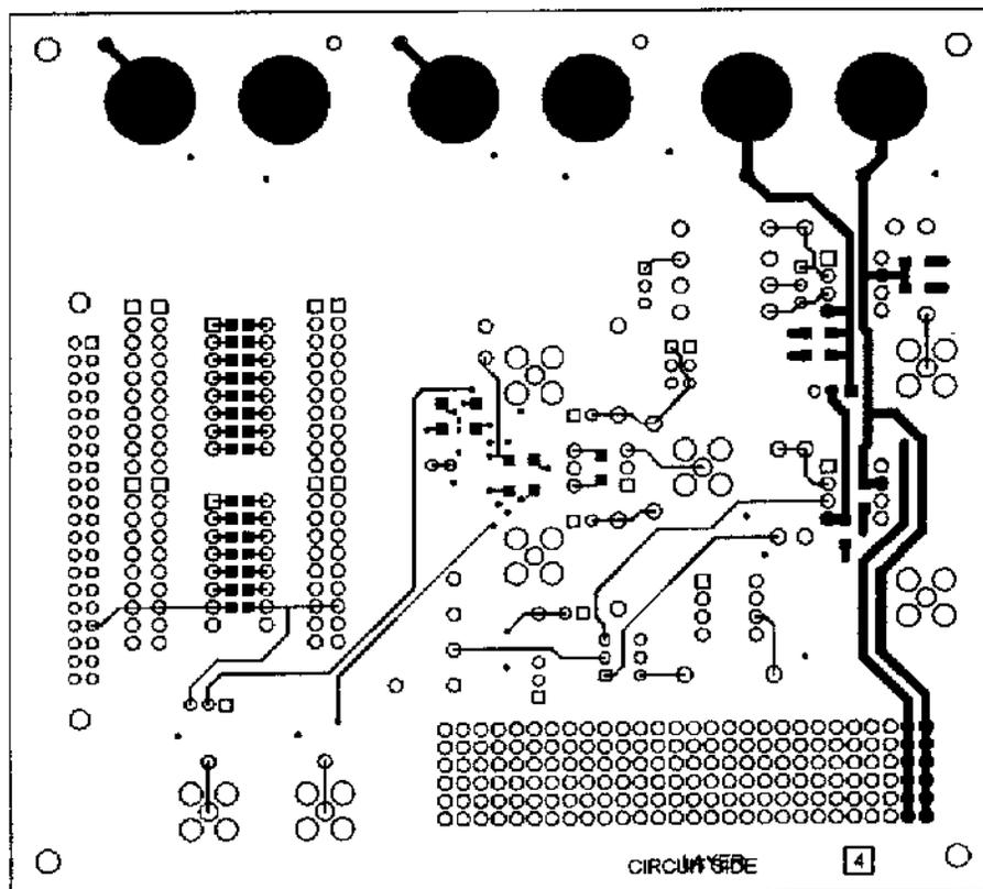
Figure 31. Solder Side PCB Layout (Layer 4)
