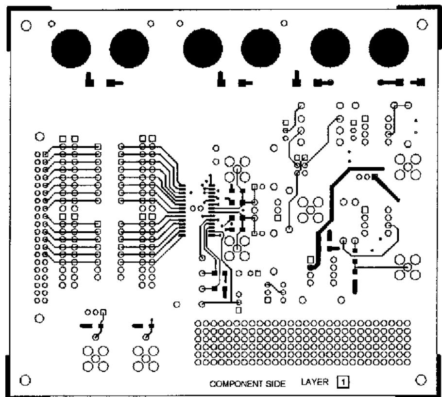
Figure 28. Component Side PCB Layout (Layer 1)
