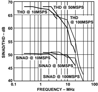
Figure 3. SINAD/THD vs.  $f_{OUT}$  (AVDD and DVDD = 5.0 V)
