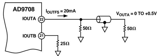
Figure 16. 0 V to +0.5 V Unbuffered Voltage Output
