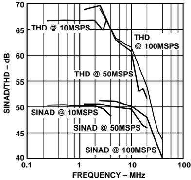
Figure 6. SINAD/THD vs.  $f_{OUT}$  (AVDD and DVDD = 3.0 V)
