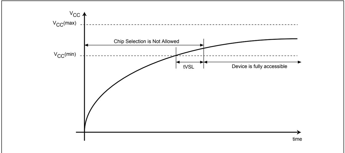
**Note:** VCC (max.) is 3.6V and VCC (min.) is 2.7V.
