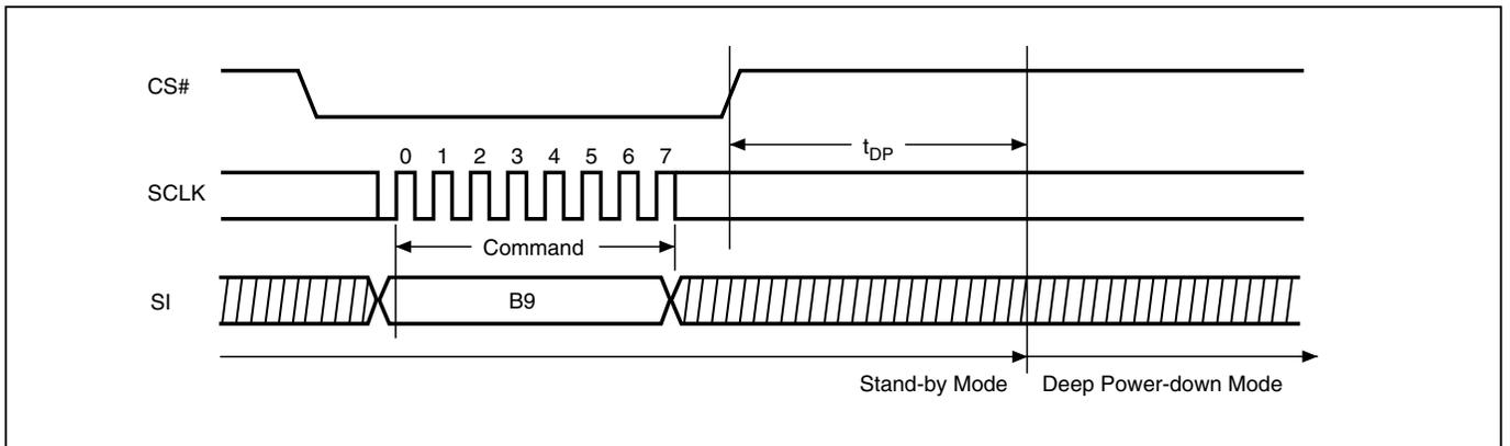
**Figure 33. Read Electronic Signature (RES) Sequence (Command AB)**
