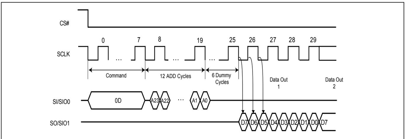
**Figure 19. 2 x I/O Read Mode Sequence (Command BB)**
