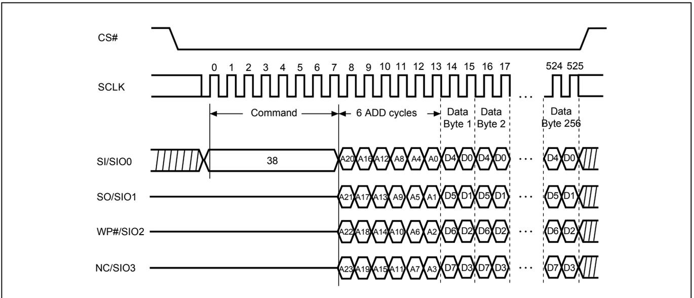
**Figure 30. Continously Program (CP) Mode Sequence with Hardware Detection (Command AD)**
