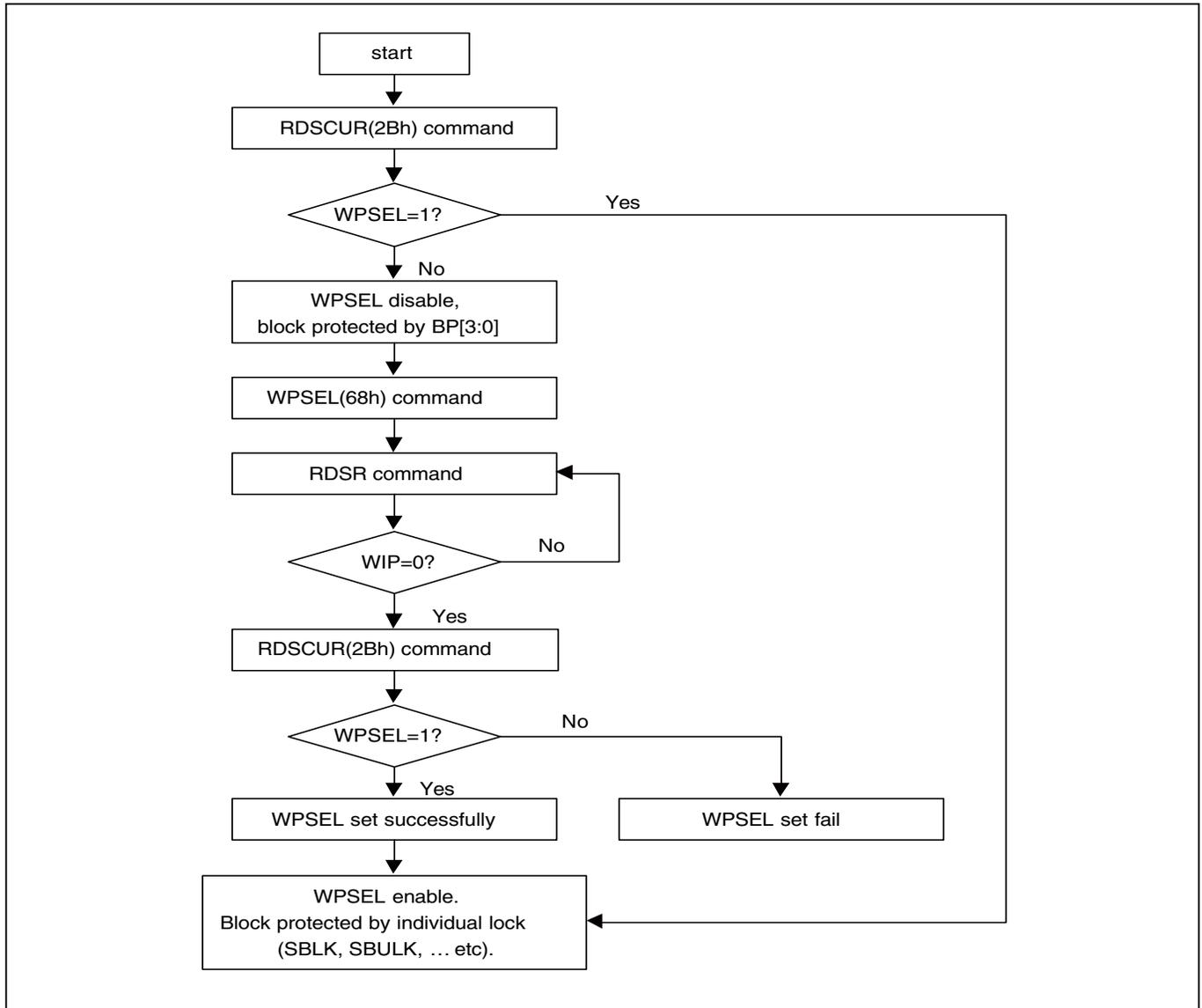
**(29) Single Block Lock/Unlock Protection (SBLK/SBULK)**
