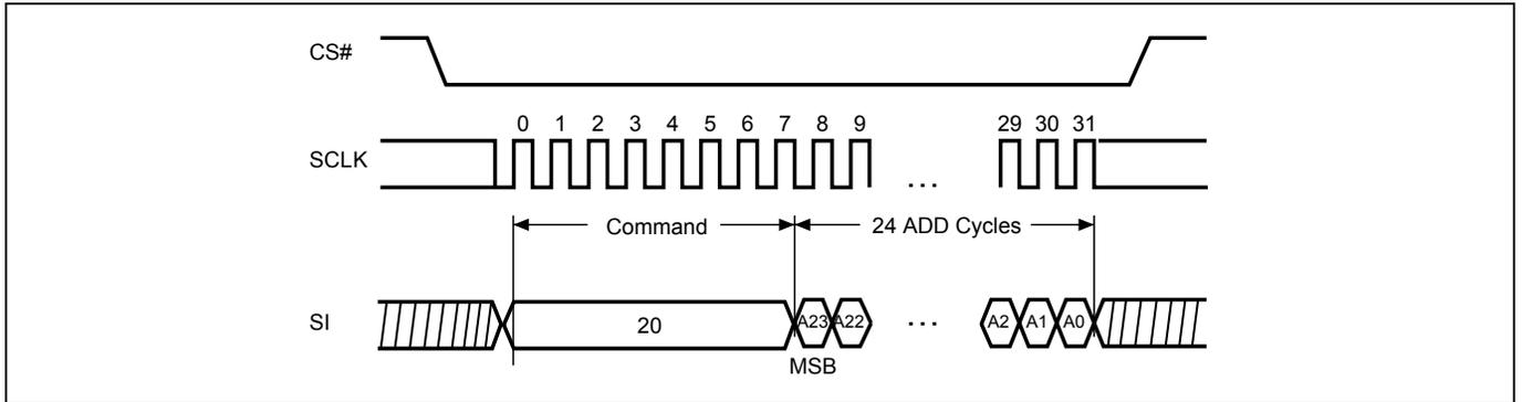
**Figure 26. Block Erase (BE/BE32K) Sequence (Command D8/52)**
