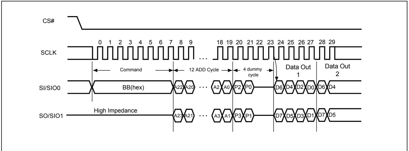
**Note:** SI/SIO0 or SO/SIO1 should be kept "0h" or "Fh" in the first two dummy cycles. In other words, P2=P0 or P3=P1 is necessary.
