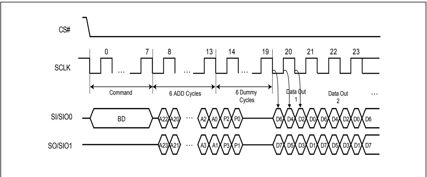
**Note:** SI/SIO0 or SO/SIO1 should be kept "0h" or "Fh" in the first two dummy cycles. In other words, P2=P0 or P3=P1 is necessary.
