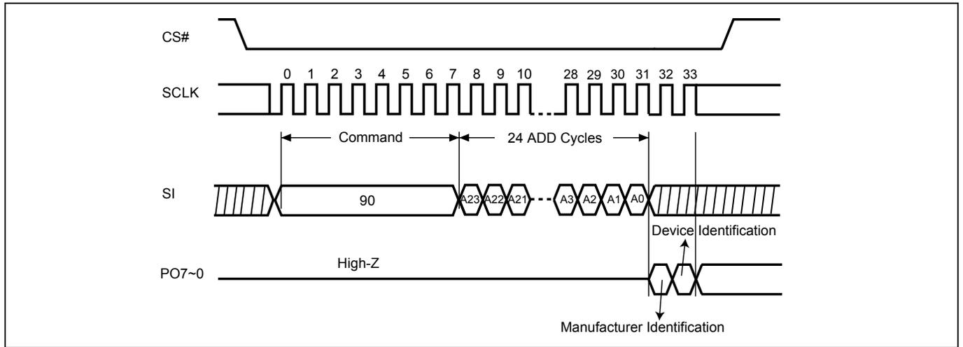
Note: A0=0 will output the Manufacturer ID first and A0=1 will output Device ID first. A1~A23 don't care.
