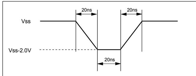
**Figure 3. Maximum Positive Overshoot Waveform**
