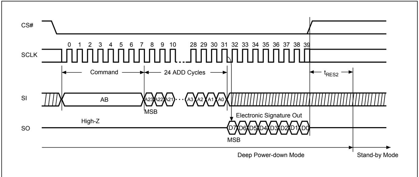
**Figure 34. Release from Deep Power-down (RDP) Sequence (Command AB)**
