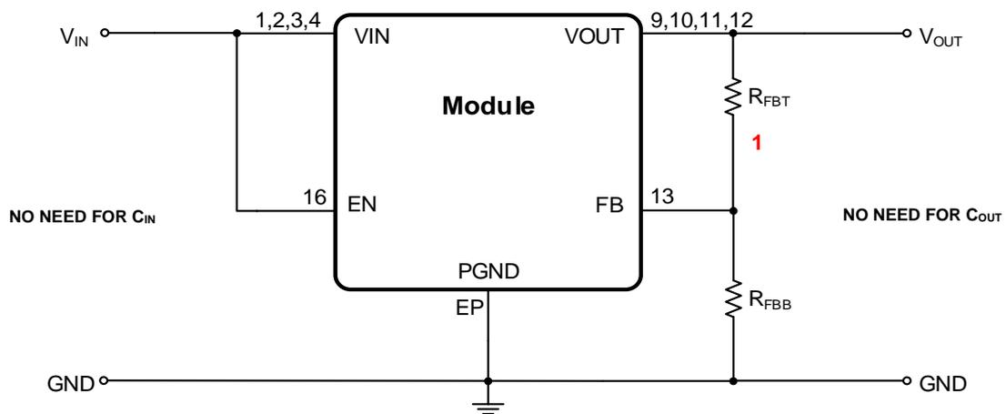
**Step 1 Set the output voltage (V<sub>OUT</sub>)**
