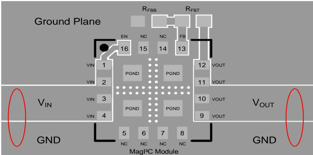
This reduces any voltage drops on the input or output of the converter and maximizes efficiency.
