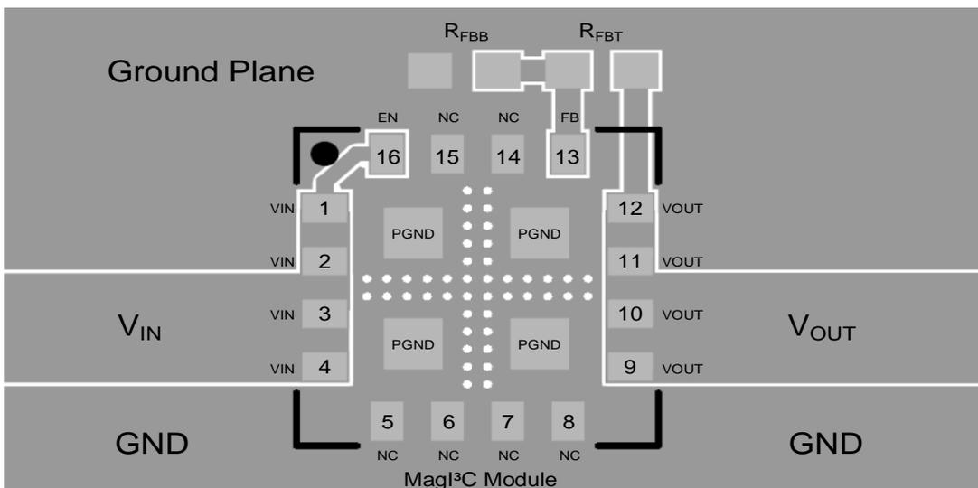
The ground connection of the lower resistor of the output voltage divider ( $R_{FBB}$ ) should be routed to the PGND pins of the device. If not properly handled, poor grounding can result in degraded load regulation or erratic output voltage ripple behaviour.
