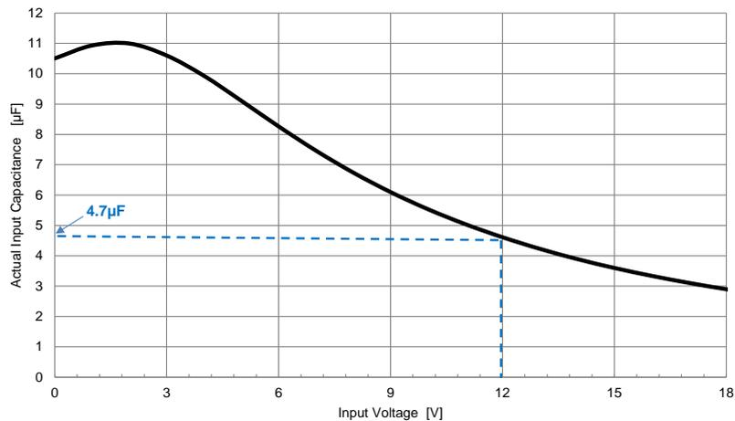
From the diagram above, the actual capacitance value of 4.7µF can be read.
