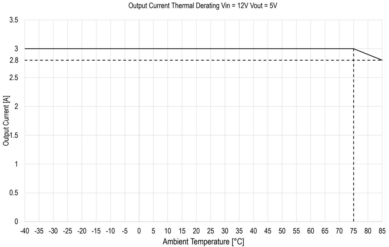
The ambient temperature and the power limits of the derating curve represent the operation at the max junction temperature specified in the “[Operating Conditions](#)” section on page 4.
