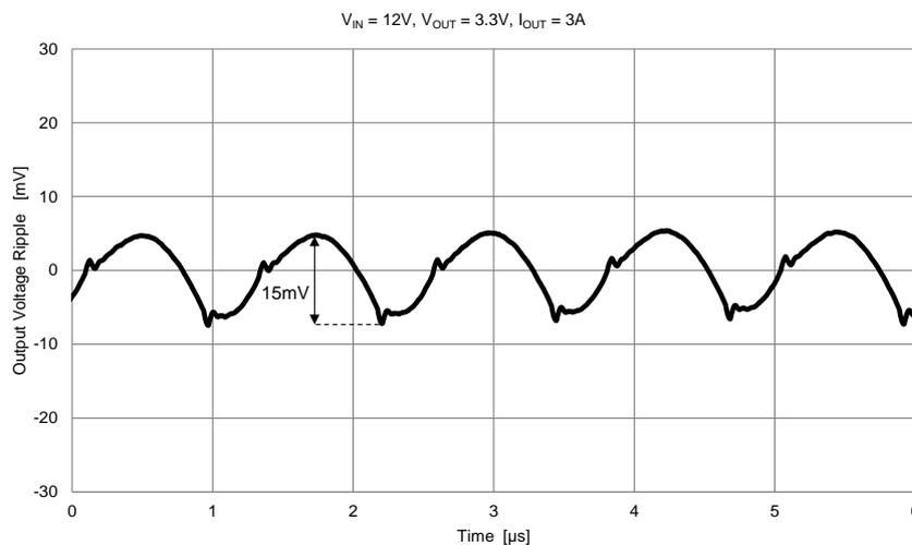
In case the application has more demanding requirements in terms of output voltage ripple, additional external capacitors should be used. The value of the external additional capacitance ( $C_{OUT,INT}$ ) can be calculated using the following equation:
