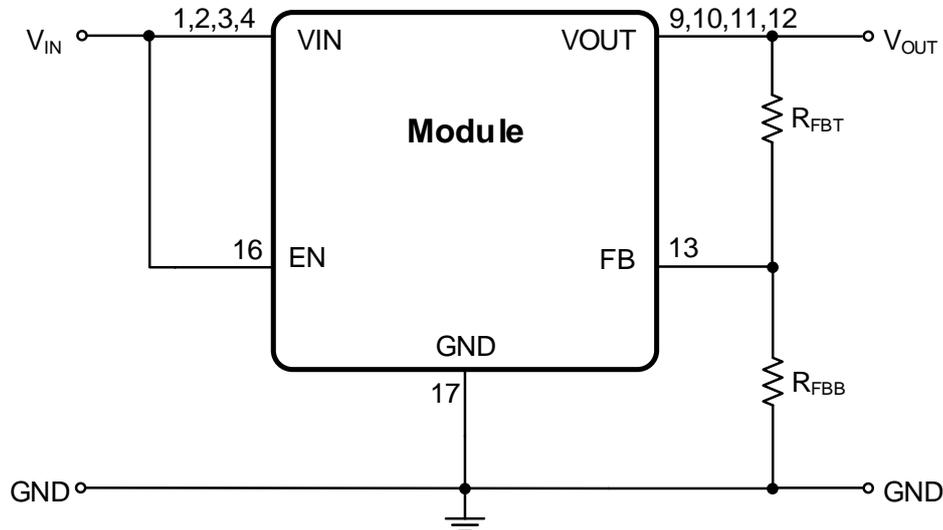
**Quick setup guide**Conditions: T<sub>A</sub> = 25°C, I<sub>OUT</sub> = 3A
