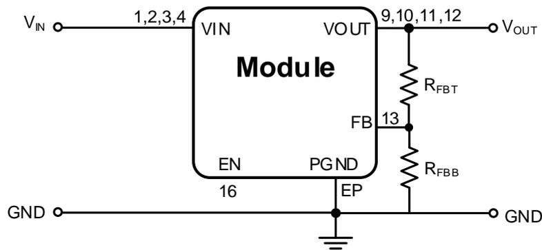
The only external components necessary to operate the 171031801 that must be placed on the PCB are the resistors of the output voltage divider, as shown in the picture above.
