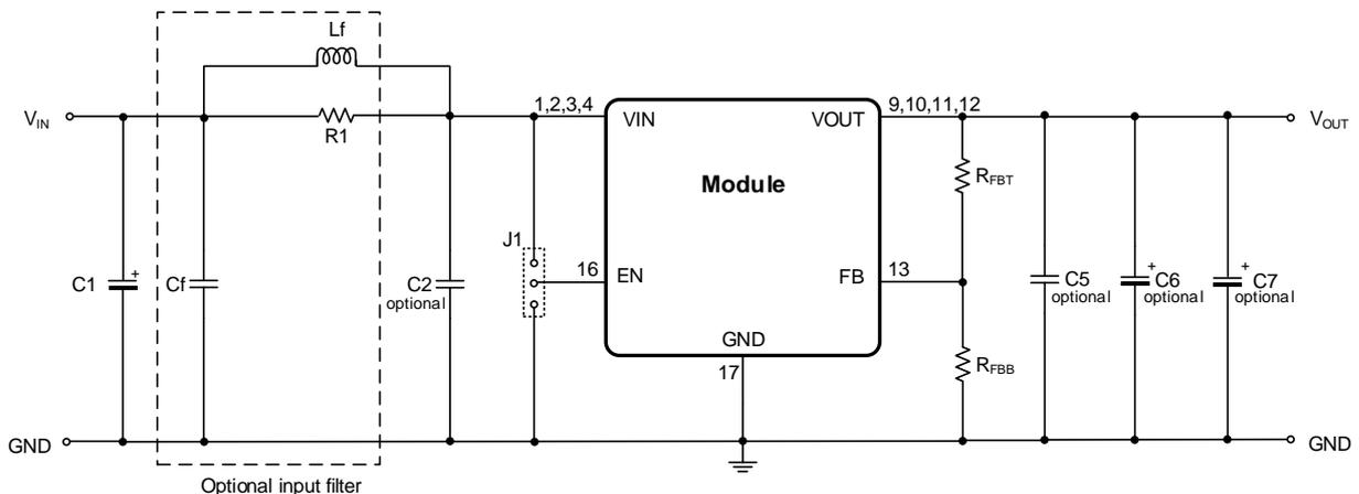
The 171031801 integrates both the input and output capacitors. Therefore, additional external input/output capacitors are normally not required.
