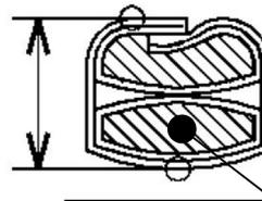
Put the smaller wire underneath
