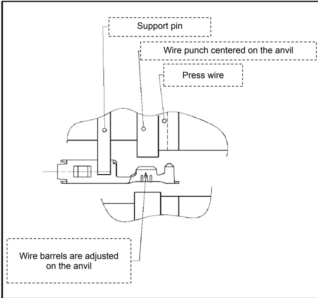
Figure 6a – TERMINAL POSITION IN TOOL
