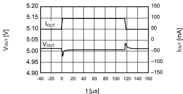
**(3) ON/OFF pin transient response characteristics**
