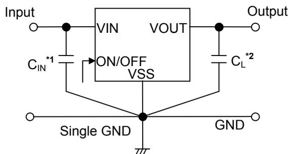
\*1.  $C_{IN}$  is a capacitor for stabilizing the input.
