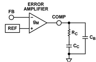
Figure 24. Compensation Components
