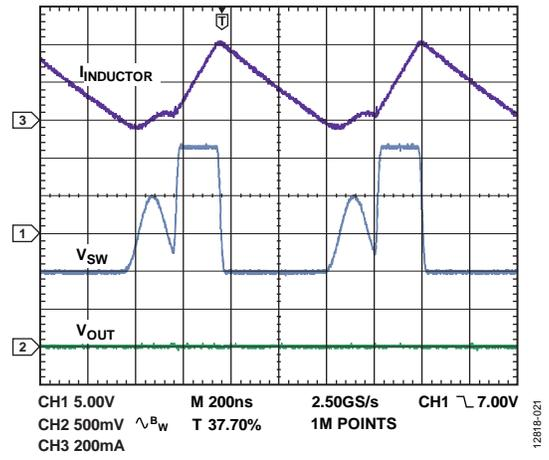
Figure 19. Discontinuous Conduction Mode Operation Showing Inductor Current ( $I_{INDUCTOR}$ ), Switch Node Voltage ( $V_{SW}$ ), and Output Ripple ( $V_{OUT}$ ),  $V_{IN} = 12\text{ V}$ ,  $V_{OUT} = -5\text{ V}$ ,  $I_{LOAD} = 100\text{ mA}$ ,  $f_{SW} = 1.2\text{ MHz}$ ,  $T_A = 25^\circ\text{C}$
