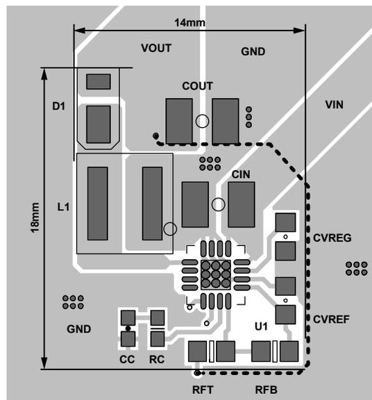
Figure 26. Suggested Layout for 18 mm × 14 mm, +12 V Input to -5 V Output Application
