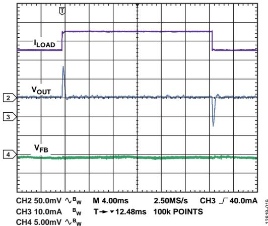
Figure 17. Load Transient Showing  $I_{LOAD}$ ,  $V_{OUT}$ , and  $V_{FB}$ ,  $V_{IN} = 12\text{ V}$ ,  $V_{OUT} = -5\text{ V}$ ,  $I_{LOAD} = 35\text{ mA}$  to  $45\text{ mA}$  Step,  $f_{SW} = 1.2\text{ MHz}$ ,  $T_A = 25^\circ\text{C}$
