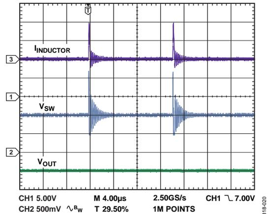
Figure 18. Skip Mode Operation Showing Inductor Current ( $I_{INDUCTOR}$ ), Switch Node Voltage ( $V_{SW}$ ), and Output Ripple ( $V_{OUT}$ ),  $V_{IN} = 12\text{ V}$ ,  $V_{OUT} = -5\text{ V}$ ,  $I_{LOAD} = 1\text{ mA}$ ,  $f_{SW} = 1.2\text{ MHz}$ ,  $T_A = 25^\circ\text{C}$
