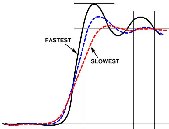
Figure 22. Switching Node at Various Slew Rate Settings
