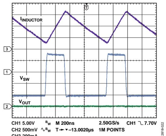
Figure 20. Continuous Conduction Mode Operation Showing Inductor Current ( $I_{INDUCTOR}$ ), Switch Node Voltage ( $V_{SW}$ ), and Output Ripple ( $V_{OUT}$ ),  $V_{IN} = 12\text{ V}$ ,  $V_{OUT} = -5\text{ V}$ ,  $I_{LOAD} = 250\text{ mA}$ ,  $f_{SW} = 1.2\text{ MHz}$ ,  $T_A = 25^\circ\text{C}$
