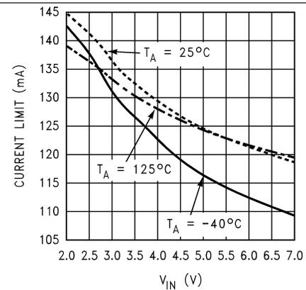
Figure 4. Switch Current Limit vs  $V_{IN}$
