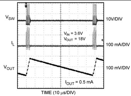
Figure 16. Output Ripple Voltage
