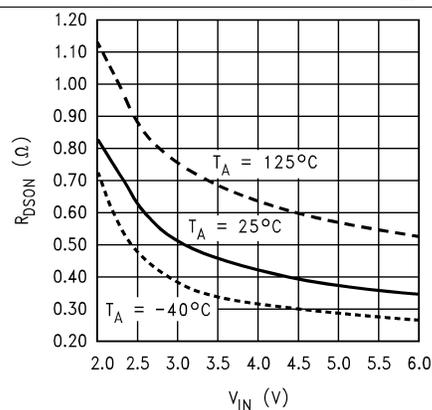
Figure 5. Switch  $R_{DS(on)}$  vs  $V_{IN}$
