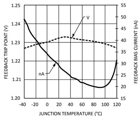
Figure 6. FB Trip Point and FB Pin Current vs Temperature
