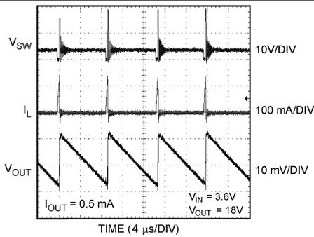
Figure 15. Output Ripple Voltage
