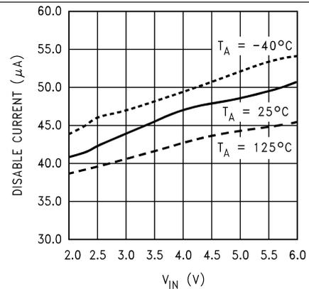
Figure 2. Disable Current vs  $V_{IN}$  (Device Not Switching)
