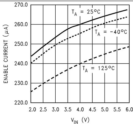
Figure 1. Enable Current vs  $V_{IN}$  (Device Switching)
