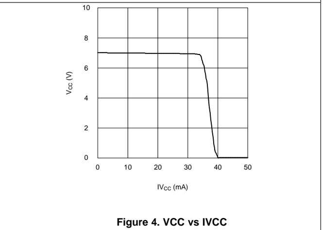
Figure 4. VCC vs IVCC
