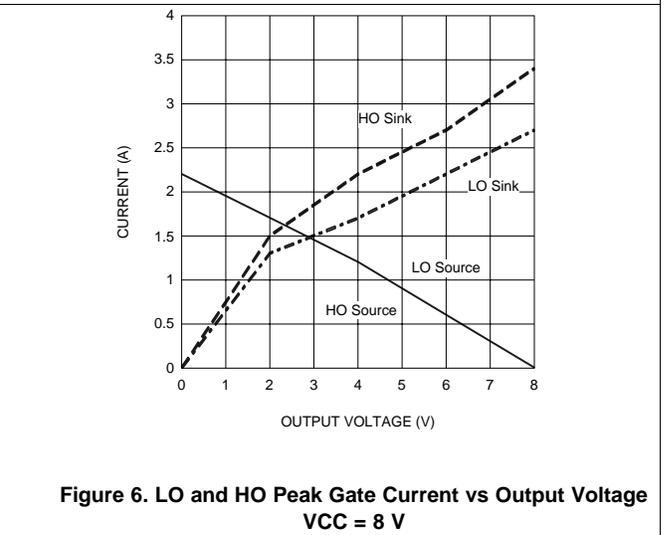
Figure 6. LO and HO Peak Gate Current vs Output Voltage VCC = 8 V
