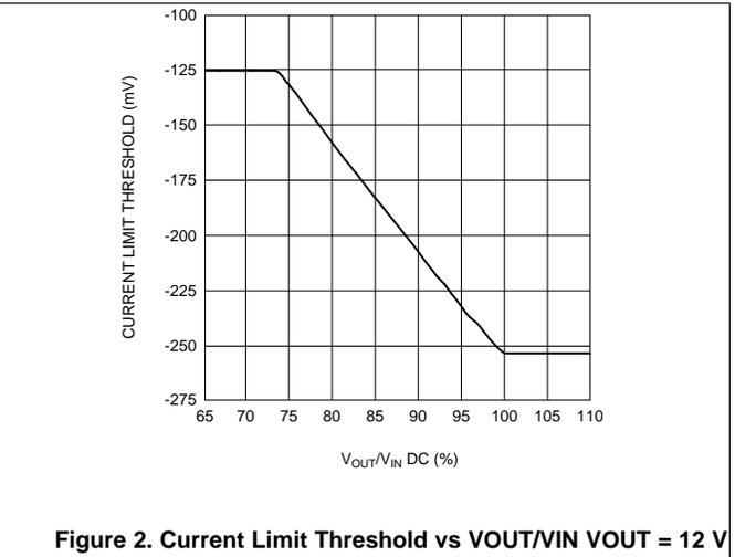
Figure 2. Current Limit Threshold vs VOUT/VIN VOUT = 12 V
