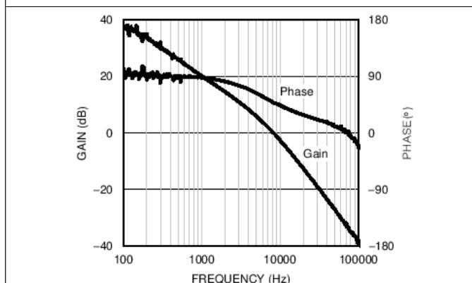
Figure 25. Overall Loop Gain and Phase - Buck Mode
