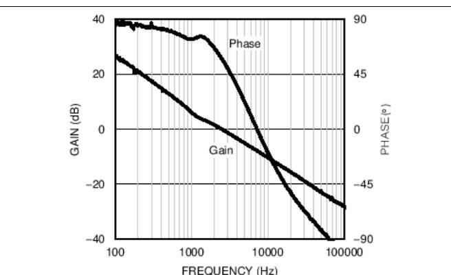
Figure 26. Overall Loop Gain and Phase - Buck-Boost Mode
