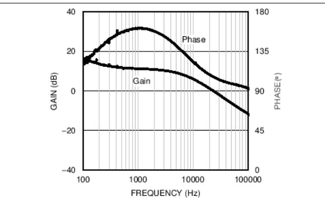
Figure 24. Error Amplifier Gain and Phase - Buck-Boost Mode
