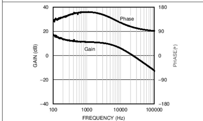
Figure 23. Error Amplifier Gain and Phase - Buck Mode
