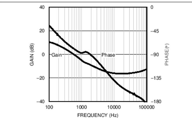
Figure 22. Modulator Gain and Phase - Buck-Boost Mode
