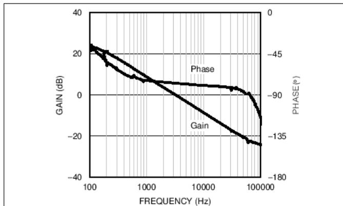
Figure 21. Modulator Gain and Phase - Buck Mode
