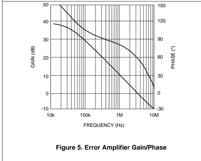
Figure 5. Error Amplifier Gain/Phase
