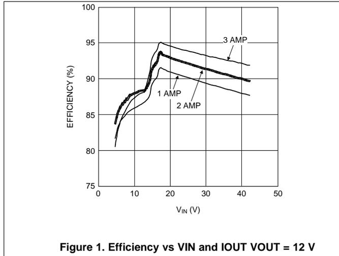
Figure 1. Efficiency vs VIN and IOUT VOUT = 12 V
