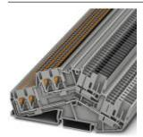
Double-level terminal block, With equipotential bonder, Cross section: 0.14 mm² - 4 mm², AWG: 26 - 12, Connection type: Push-in connection, Width: 5.2 mm, Color: gray, Mounting type: NS 35/7,5, NS 35/15
