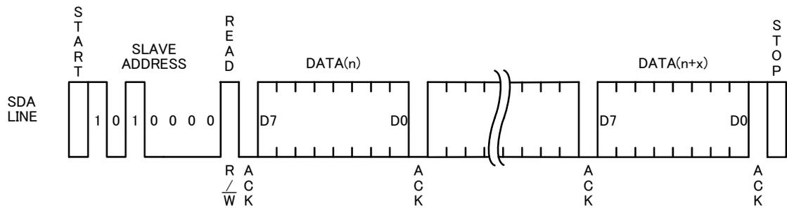
Fig.-12 SEQUENTIAL READ CYCLE TIMING
