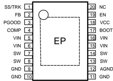
**Figure 1. 20-Pin HTSSOP, Top View**
