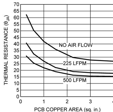
**Figure 32. Thermal Resistance vs PCB Area (4 Layer Board)**
