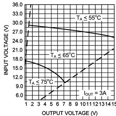
**Figure 30. Safe Thermal Operating Areas ( $I_{OUT} = 3A$ )**
