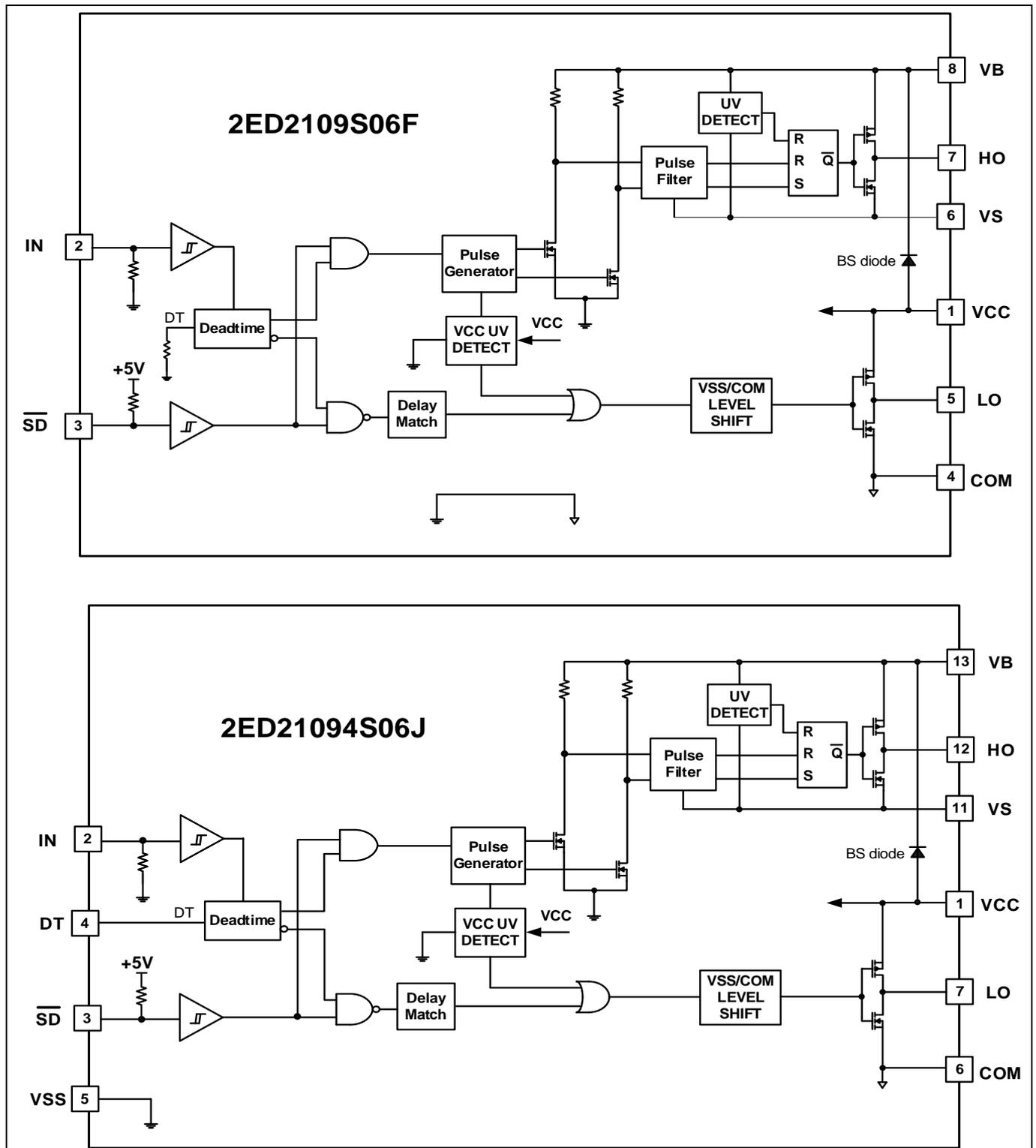
Figure 2 Block diagrams
