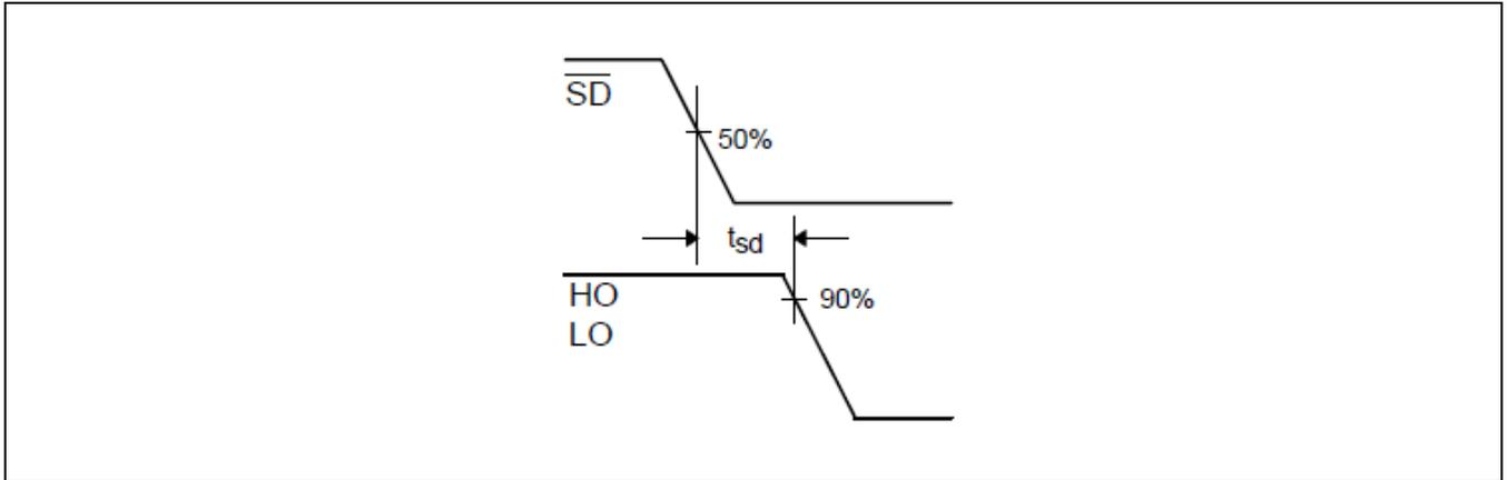
Figure 12 Shutdown waveform definitions
