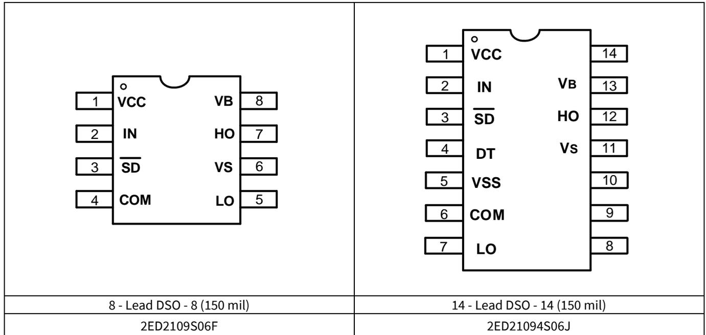
Figure 3 2ED2109 (4) S06 F(J) pin assignments (top view)
