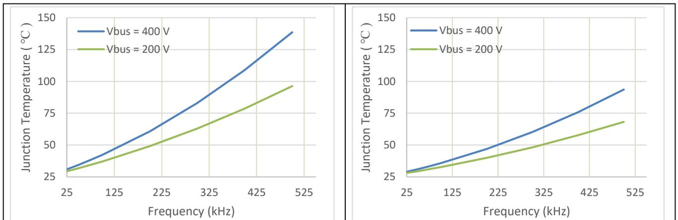
\*Assumptions for above curves: LLC topology, Power switch = IPP60R600P6,  $T_a = 25\text{ °C}$ ,  $V_{BUS} = 400\text{ V}$ ,  $V_{CC} = 12\text{ V}$ ,  $R_{gon} = 3.9\ \Omega$ ,  $R_{goff} = 1\ \Omega$
