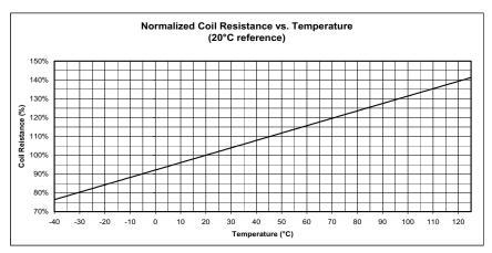
Example: Resistance of  $100\Omega$  coil = 75% of  $100\Omega$  at  $-40^{\circ}$ C, or  $75\Omega$  = 100% of  $100\Omega$  at  $20^{\circ}$ C, or  $100\Omega$  = 125% of  $100\Omega$  at  $85^{\circ}$ C, or  $125\Omega$
