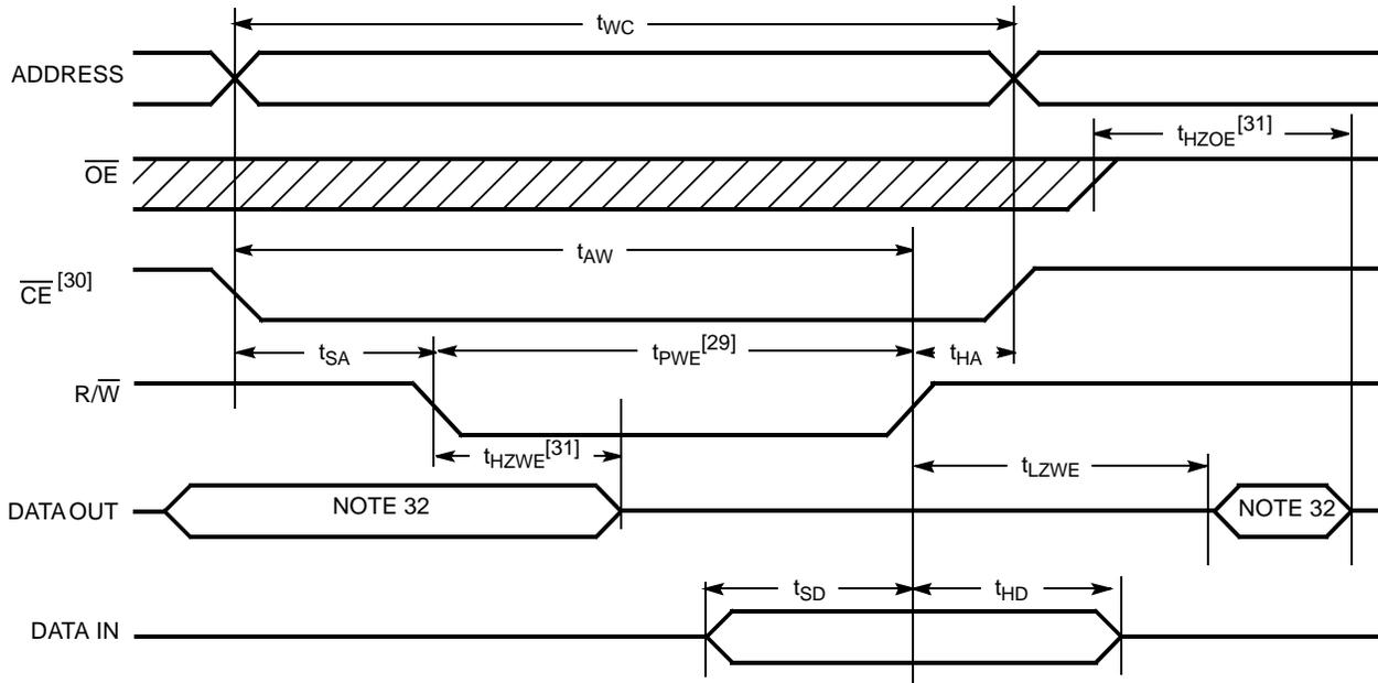
**Write Cycle No. 2: CE Controlled Timing<sup>[26, 27, 28, 33]</sup>**
