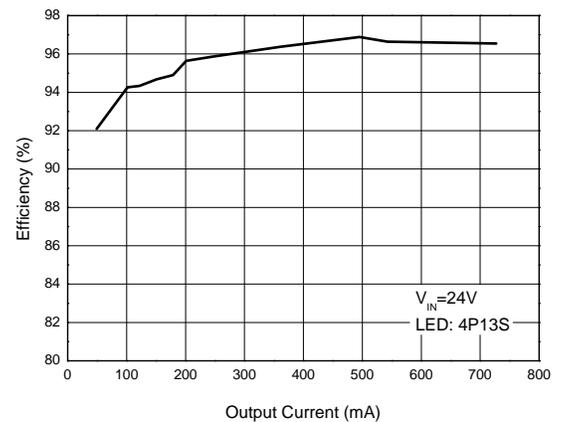
**Performance Characteristics** (Cont.  $V_{IN}=24V$ ,  $V_{EN}=V_{DD}=5V$ , 13 LEDs in series, 4 strings in parallel, 120mA/string,  $T_A=+25^{\circ}C$ , unless otherwise specified.)
